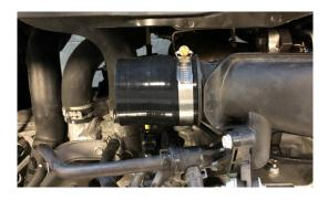
12. INSTALL MAF ON TO INTAKE USING INCLUDED HARDWAREV
