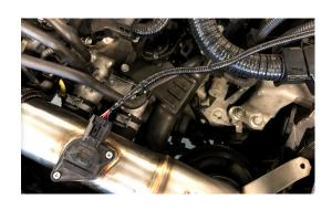
16. INSTALL INCLUDED BOLT ONTO SUPPORT TAB, THIS WILL THREAD INTO AN EXISTING AIR BOX BRACKET ON THE CAR
