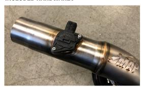
13. INSTALL INTAKE INTO THE COUPLER AND TIGHTEN BOTH CLAMPS
