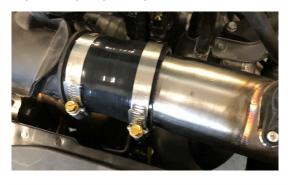
14. REMOVE THE MAF WIRING ELBOW CLAMP, SLIDE CORRUGATED WIRING COVER BACK, USE ELECTRICAL TAPE TO SECURE AND COVER ANY EXPOSED WIRING
