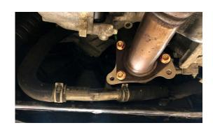
13. REINSTALL DOWNPIPE BRACKET AND BOLTS
