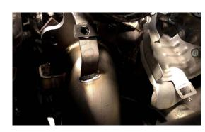
10-3. SLIDE OEM HEAT SHIELD IN THE THROUGH THE BOTTOM
