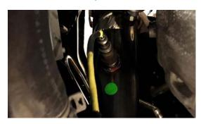
10A-D. INSTALL NEW DOWNPIPE, REPLACE THE USED NUTS WITH INCLUDED HARDWARE AND REINSTALL BOLTS. BE SURE THE GASKET IS IN PLACE AND ALL NUTS AND BOLTS ARE TIGHT
