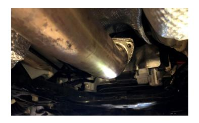
5A-B. INSTALL MID PIPE FRONT CONNECTION TO THE FRONT PIPE, BE SURE GASKET IS INSTALLED AND NUTS ARE TIGHTENED
