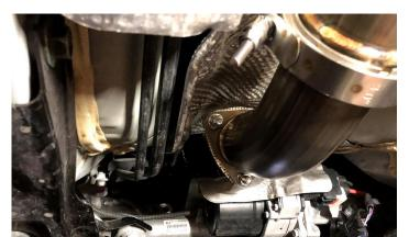
15. REINSTALL THE 4 10MM BOLTS HOLDING THE SPLASH GUARD UP IN THE REAR
