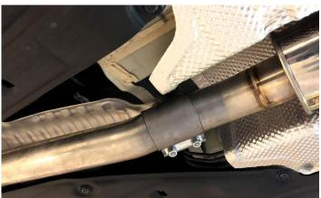
13. GO THROUGH AND CLOCK ALL SECTIONS OF THE CAT BACK ENSURING IT IS NOT BOUND UP OR HANGING IN THE WRONG POSITION. IT SHOULD SIT HOW IT APPEARS IN THE PICTURES
