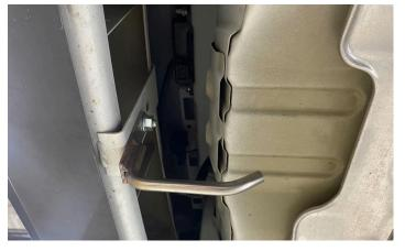
8B. INSTALL ON OF OUTER OEM MUFFLER RUBBER HANGER, INSTALLED AS PICTURED
