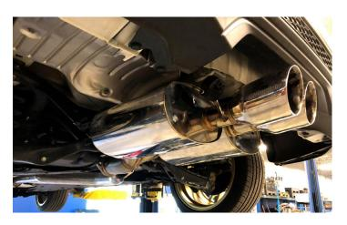
3A-B. REMOVE 3 NUTS HOLDING THE FRONT PIPE TO THE AXLE BACK
