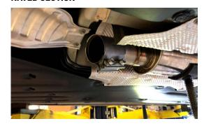
11. INSTALL REAR SECTION OF RESONATED PIPE ONTO MUFFLER LOOSELY WITH V-BAND CLAMP
