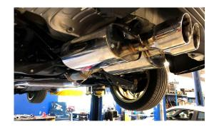
3. REMOVE 3 NUTS HOLDING THE FRONT PIPE TO THE AXLE BACK
