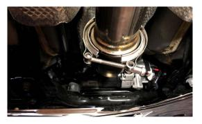
8. INSTALL RUBBER HANGERS ONTO MUFFLER SECTION (THESE SHOULD ALSO BE REMOVED FROM YOUR FACTORY EXHAUST)
