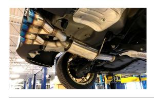
10. INSTALL SLIP CLAMP ONTO FRONT RESONATED SECTION
