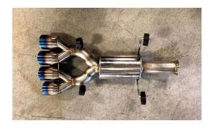
9. INSTALL MUFFLER SECTION ONTO THE BODY
