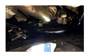
4. REMOVE REMAINING RUBBER HANGER AND REMOVE THE REST OF THE EXHAUST
