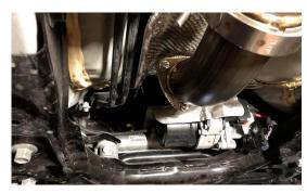
15. REINSTALL THE 4 10MM BOLTS HOLDING THE SPLASH GUARD UP IN THE REAR
