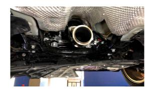
6. INSTALL RUBBER HANGER ONTO (FROM YOUR OLD AXLE BACK) ONTO YOUR NEW AXLE BACK RESONATED PORTION
