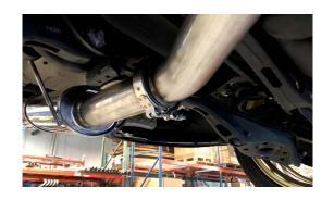
12. SLIDE SLIP CLAMP ONTO REAR SECTION OF THE RESONATED PIPE, SNUG THE CLAMP UP BUT BE SURE IT CAN STILL MOVE SLIGHTLY
