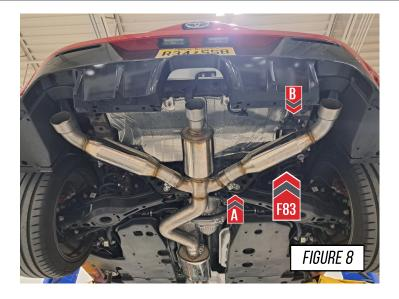
To install the exhaust tips with integrated clamps, first, attach the exhaust tip in the proper orientation onto the exhaust outlet tube.
