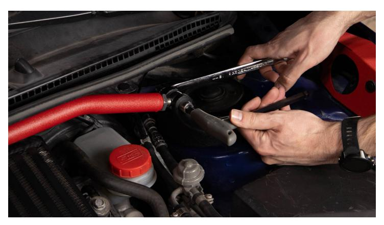
Step 6 - Tighten down the locking nut. Snug is good here but if you have a crows foot, torque to 35 Ft/Lbs.
