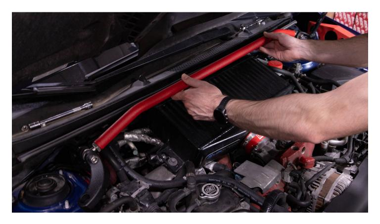
Step 4 - Reinstall the nuts one each side, torque to 14.8 Ft/Lbs.
