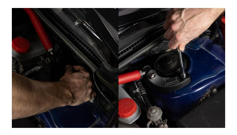
Step 5 - Using a 10mm Hex bit and 18mm wrench tighten the nut and bolt to 35 Ft/Lbs.
