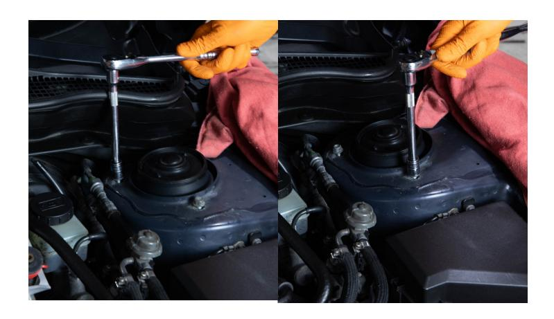
Step 3 - Take your GrimmSpeed Strut Bar and align the holes in the mounts with the two studs.
