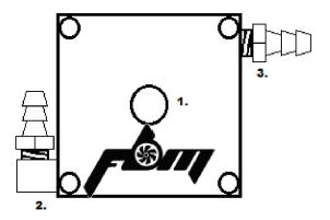
The can mounts to firewall, onto an existing stud. Attach the can using the supplied bracket and M8x1.25mm nut.
