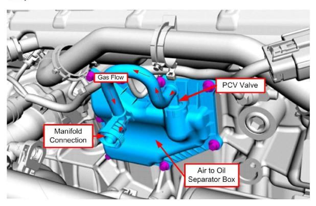
3. Route this line to the Valvecover. By applying heat to the oem plastic fitting, the plastic line can be removed without damage. Once the OEM plastic fitting has been removed, slide the supplied rubber hose on (See diagram)
