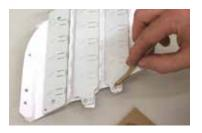
5. Fix the new panels in place by applying epoxy or other permanent adhesive where the plastic rivets were shaved down. The epoxy should create a bond between the plastic rivet point and the board. Use enough epoxy so that there is a bond all the way around the rivet, contacting the board fully.
