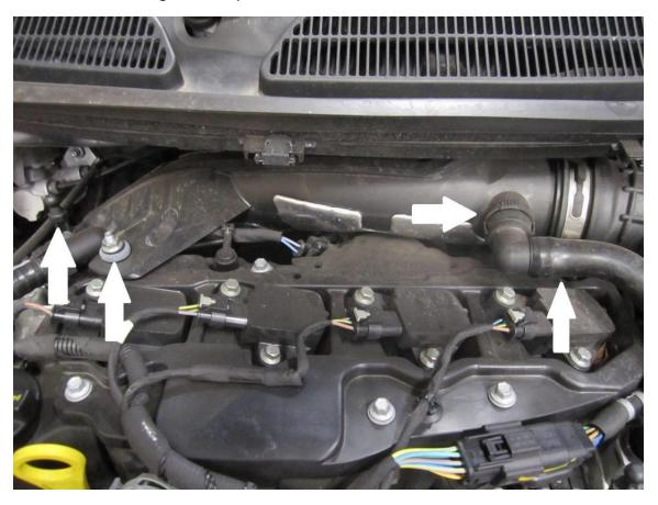
3. The plastic pipe can now be removed from the car.
