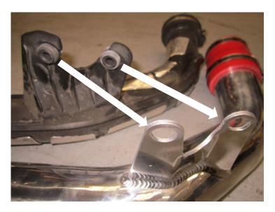
5. Fit the supplied hose to the pipe but do not tighten the clamps at this point. Ensure the hose clamps are suitably orientated for tightening on the car.
