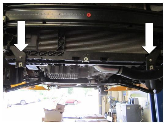
16. Now its time to fit your new forge motorsport intercooler. This is an oem fitting product, push your new intercooler into position then tighten the two m6 cap screws provided, and attach the hoses
