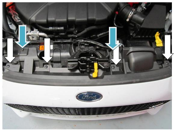
3. Using a flat headed screwdriver, or T30 torx drive, undo the two fasteners in line with the blue arrows.
