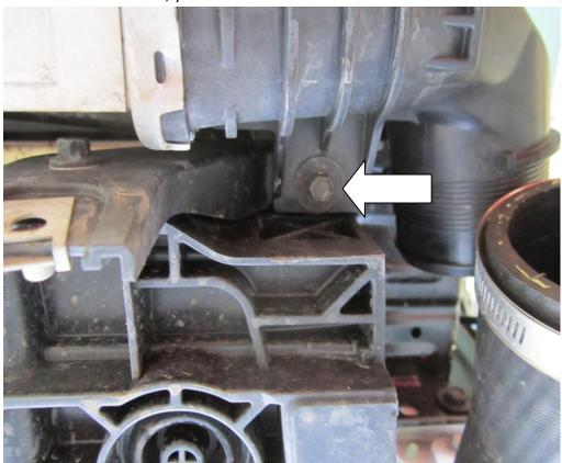
14. Remove this centre bracket from the lower ducting, it is no longer used with your new forge motorsport intercooler.
