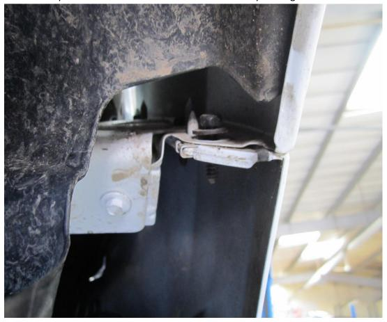
7. Once removed, pull the bumper down to release the sides. Then repeat the steps four to six on the opposite arch
