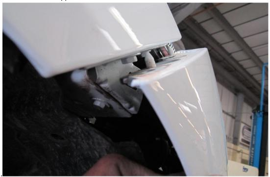
8. Two plastic fixings are on either side of the undertray. These will be found towards the rear of the undertray and must also be removed. Once these are removed carefully remove your bumper, you may want to ask for help from a friend as the fog lights will need disconnecting.
