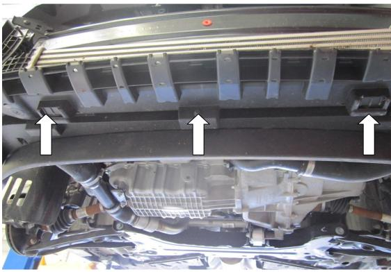
13. Undo the two fixings that mount the intercooler one on the left and one on the right. Use an 8mm socket and ratchet for this task. Slowly pull the intercooler towards you in a downward motion; your intercooler is now removed.
