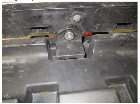
15. Remove these two fixings from the front cowling and replace with the two pan head m6 bolts provided in your forge intercooler kit
