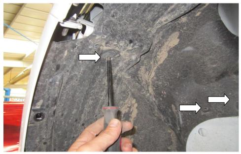
6. Pull back the arch liner; located at the inside of the bumper you will find three 10mm bolts that attach the bumper to the arch. We found it was best to use an 10mm swan neck spanner to loosen these then its best to use your fingers to remove .
