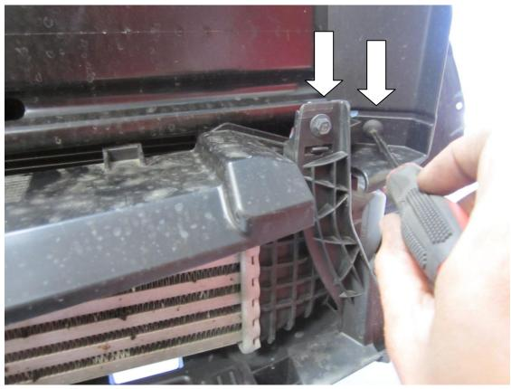
12. Now remove the lower ducting using an 8mm spanner on the three fasteners.
