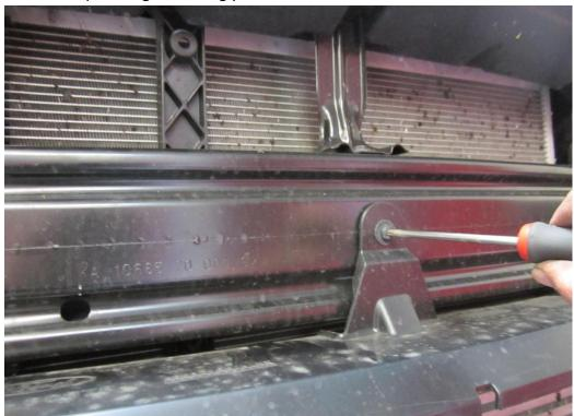
11. On each side of the top ducting there are two fasteners, use a m8 and pozi screwdriver to remove these
