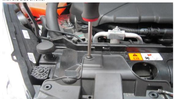
4. Now move on to the fasteners located in the wheel arch, again using either a flat bladed screwdriver or a T30 torx drive. Undo all four fixings
