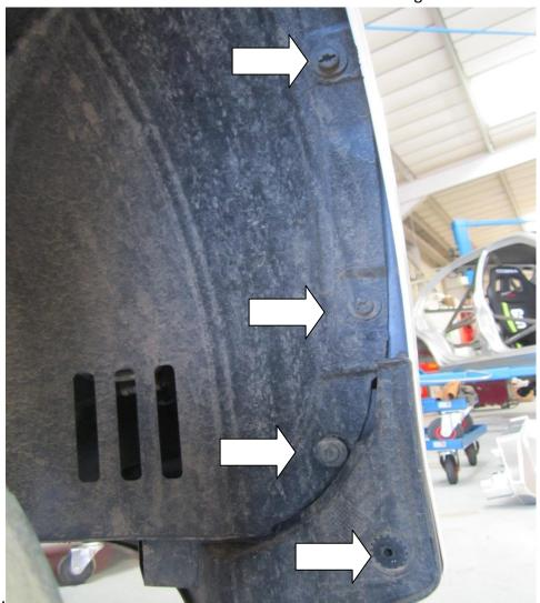
5. You will also find three plastic fasteners these can be removed with a pozi drive screwdriver.
