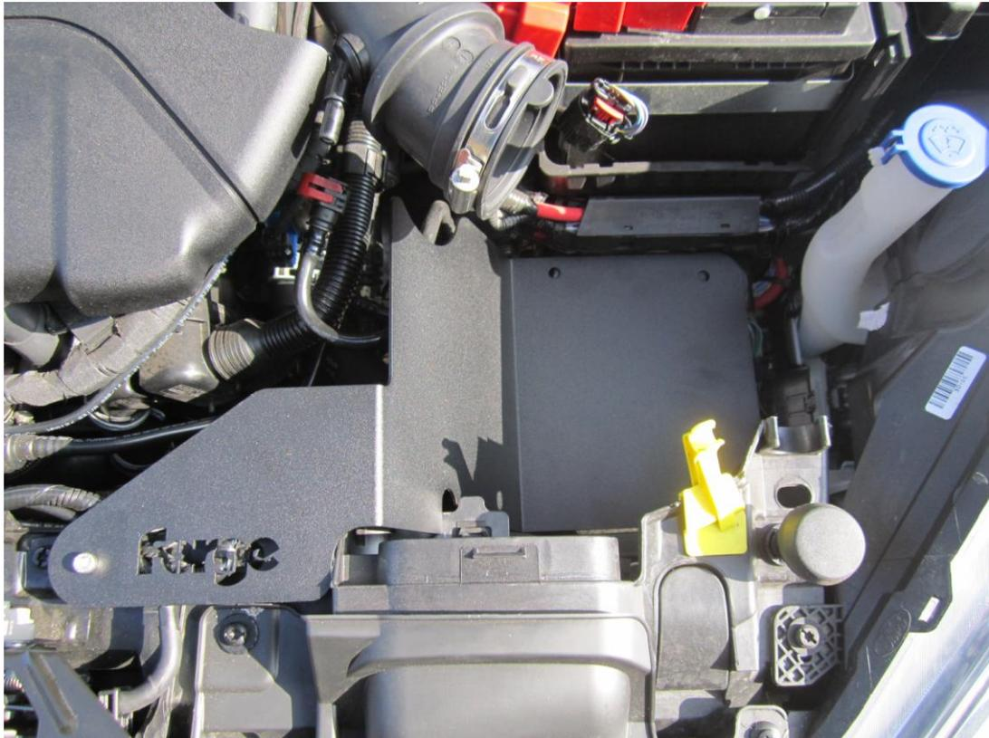
6. Using the M6 fastener provided, place the fastener through the induction tray and bolt to your slam panel .
