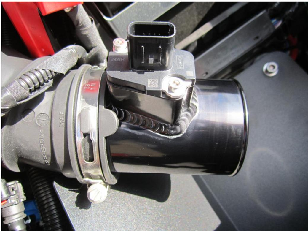
11. Now using your hose clamp driver fit the new high flow forge motorsport filter on to the end of the MAF housing .
