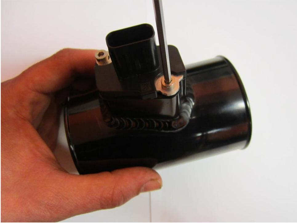
10. Now fit the MAF housing into the induction pipe making sure it is the same orientation as pictured.
