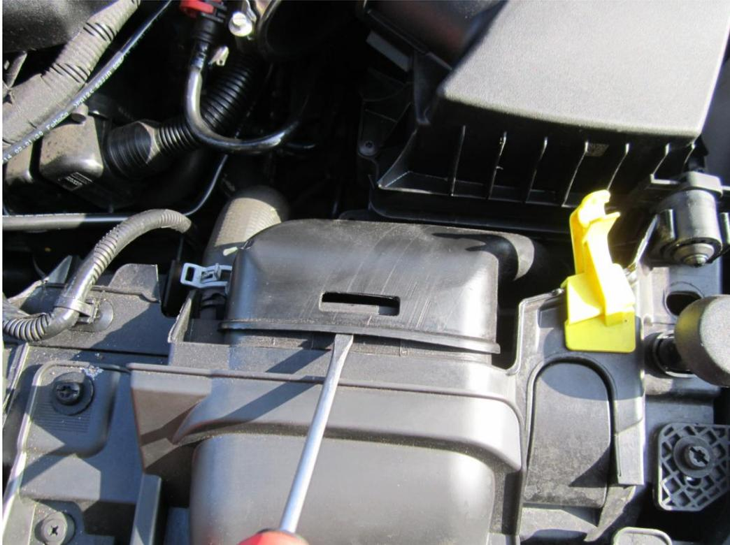
4. Now pull the airbox upwards to remove it from the rubber grommets that hold it place.
