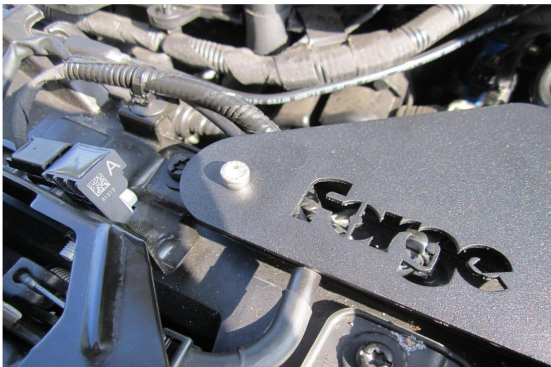
7. Using the two M8 fasteners place them through the induction tray putting the penny washers underneath followed by the two M8 nuts and secure in place.
