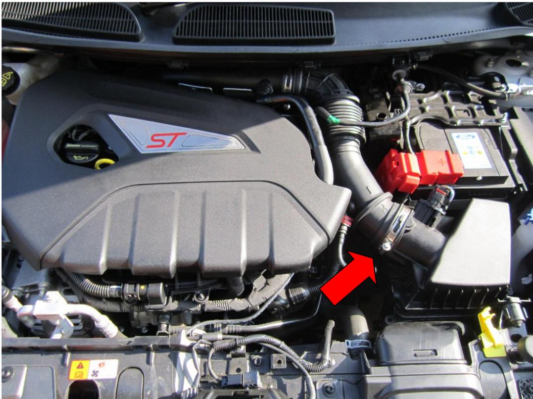
2. Now unclip the wiring loom from your MAF sensor, pull back the retaining clip that holds it in place then pull the loom away from the MAF sensor itself.
