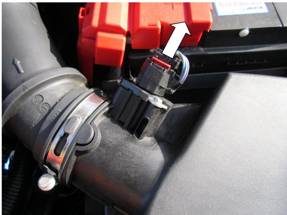
3. Using a flat bladed screwdriver pry the duct over the locator on the slam panel.
