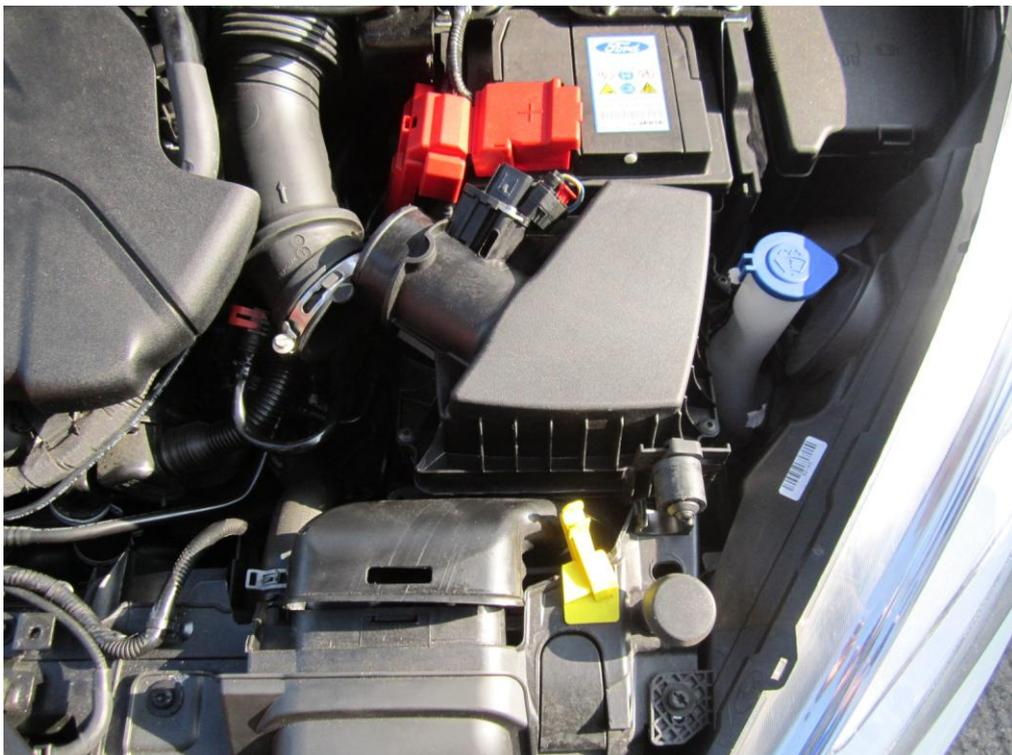
5. Now with the airbox removed place the new Forge Motorsport induction tray into position.
