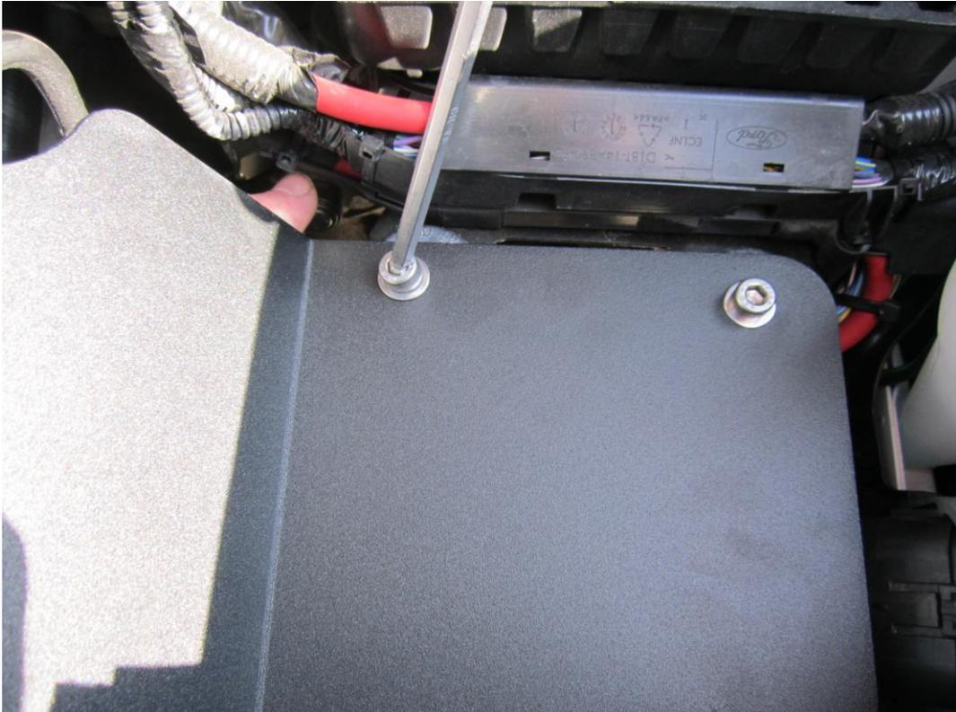
8. Using your T20 Torx drive remove the MAF sensor from your OEM airbox.
