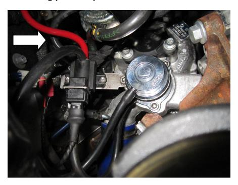
12. Using the posi locks provided attach them to the original wiring loom making sure the grey end is attached to the oe loom.
