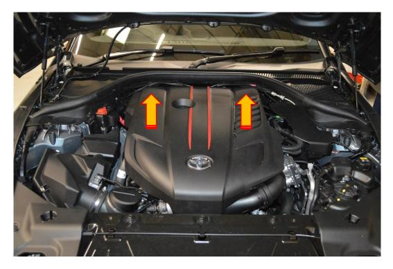
2. Next remove the vehicles air box, release the hose clamp using a 7mm socket and rachet or flat blade screwdriver. Unplug the MAF sensor by depressing the retaining clip. The air box will now pull out of the engine bay.
