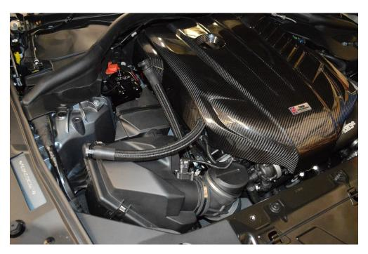
13. Fit the breather hoses to the catch can, the hose from the cam cover locates to the IN and the hose connected to the intake pipe locates to the OUT of the catch can.
