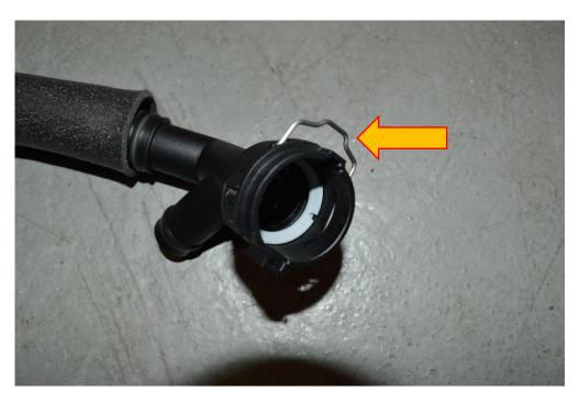
8. Insert the Forge machined breather adaptor onto the intake pipe, connect the small breather pipe to the smaller spout. Fit the LONGER hose from the FMCT6 kit with 45 degrees Norma fitting to the remaining spout.
