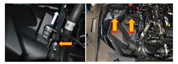
3. Locate the breather hose on top of the cam cover, squeeze the sides of the Norma fitting to release it.
