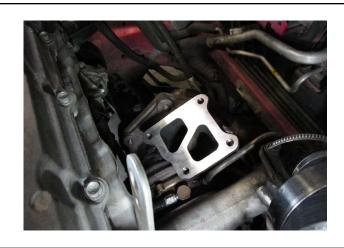
5. MAKE SURE TURBO GASKET IS ON THE HOUSING AND INSTALL THE LOWER/INNER DRIVERS SIDE BOLT FROM THE MANIFOLD TO THE TURBO FIRST, AND SNUG THE BOLT DOWN, AS OTHERWISE YOU WILL NOT BE ABLE TO GET TO IT IN THE CAR EASILY WITH ALL OTHER BOLTS IN. INSTALL THE REMAINING BOLT, AND THE TWO STUDS IN THE MANIFOLD AND TIGHTEN THEM ALL DOWN
