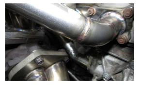
7. YOU CAN NOW INSTALL THE CAM ANGLE SENSOR HEAT SHIELD, BY REMOVING THE FACTORY LIFT HOOK AND USING THE SUPPLIED HARDWARE TO INSTALL THE SHIELD AS PICTURED
