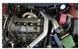
2. REMOVE TWO TURBO TO MANIFOLD NUTS, THEN TWO STUDS
