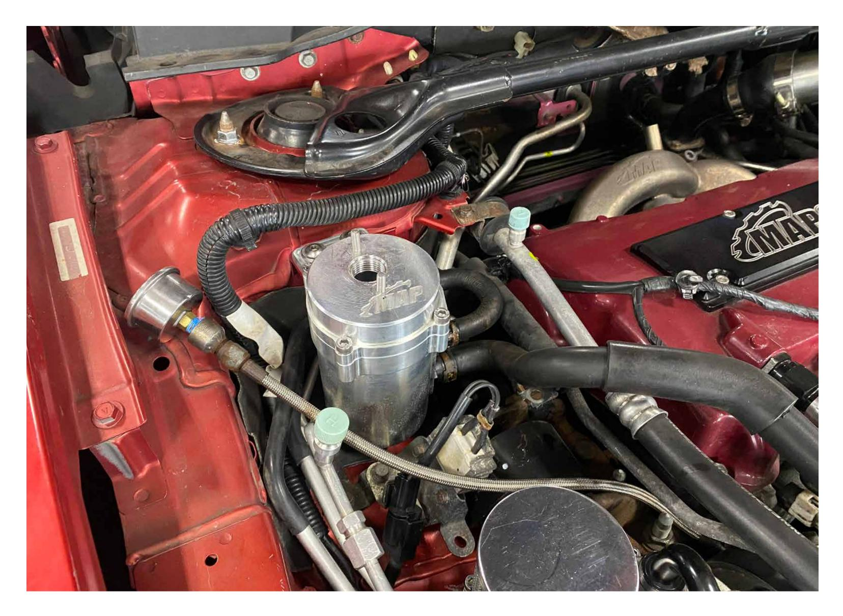
Attach MAP evox PSR to the factory reservoir mounting bracket using uncluded 5mm allen head bolts
