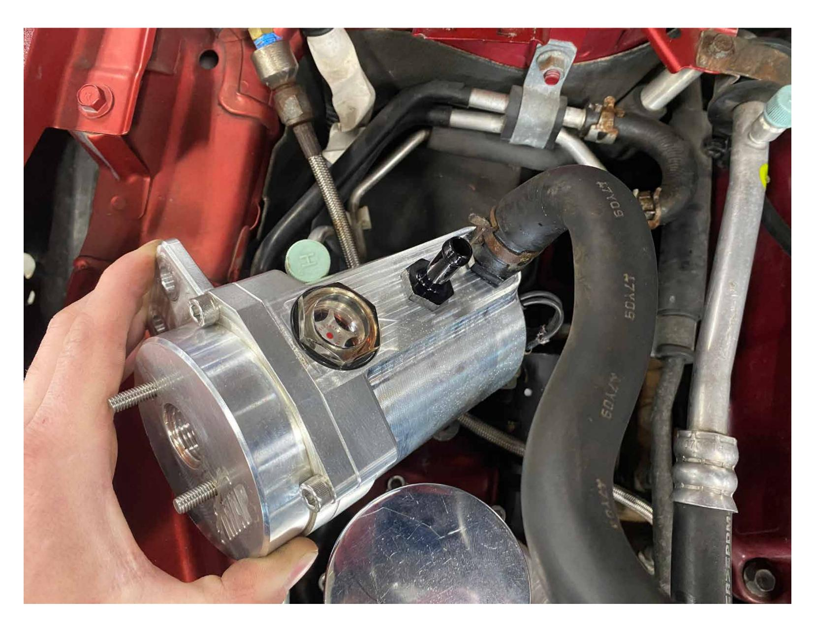
Attach lower hose to MAP evox power steering reservoir
