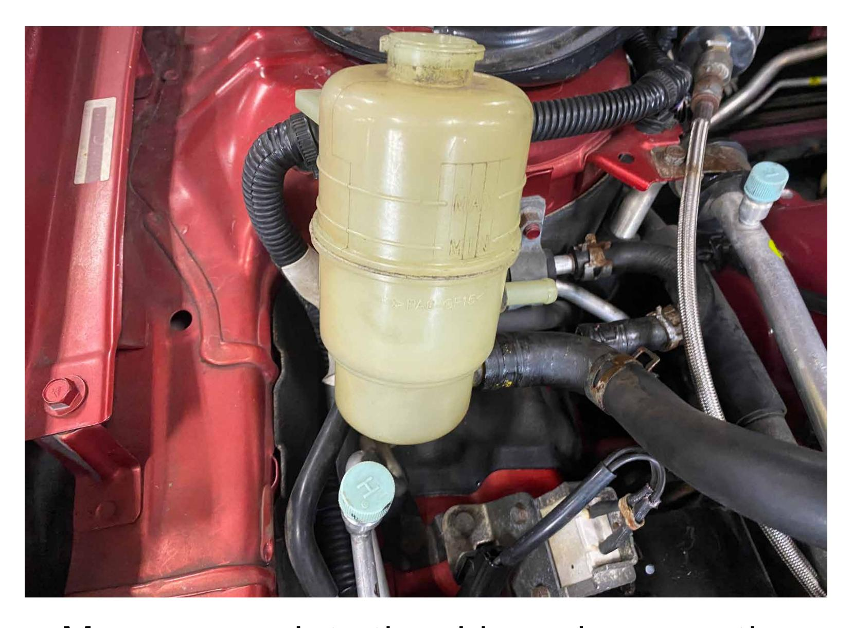
Move reservoir to the side and remove the lower hose
