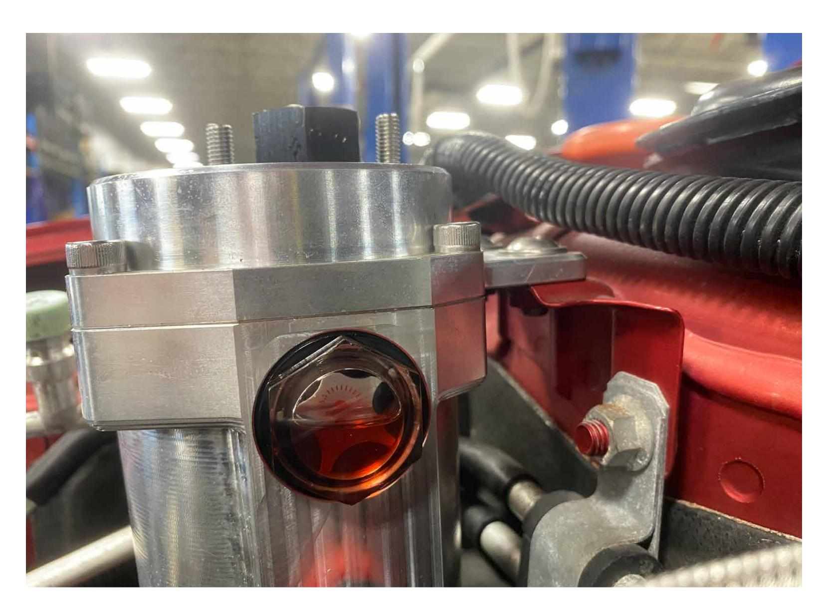
Fill PSR to the halfway point in the sightglass. It is important after install that you start the car, move the wheel side to side a few times and recheck the level to ensure the system is full.
