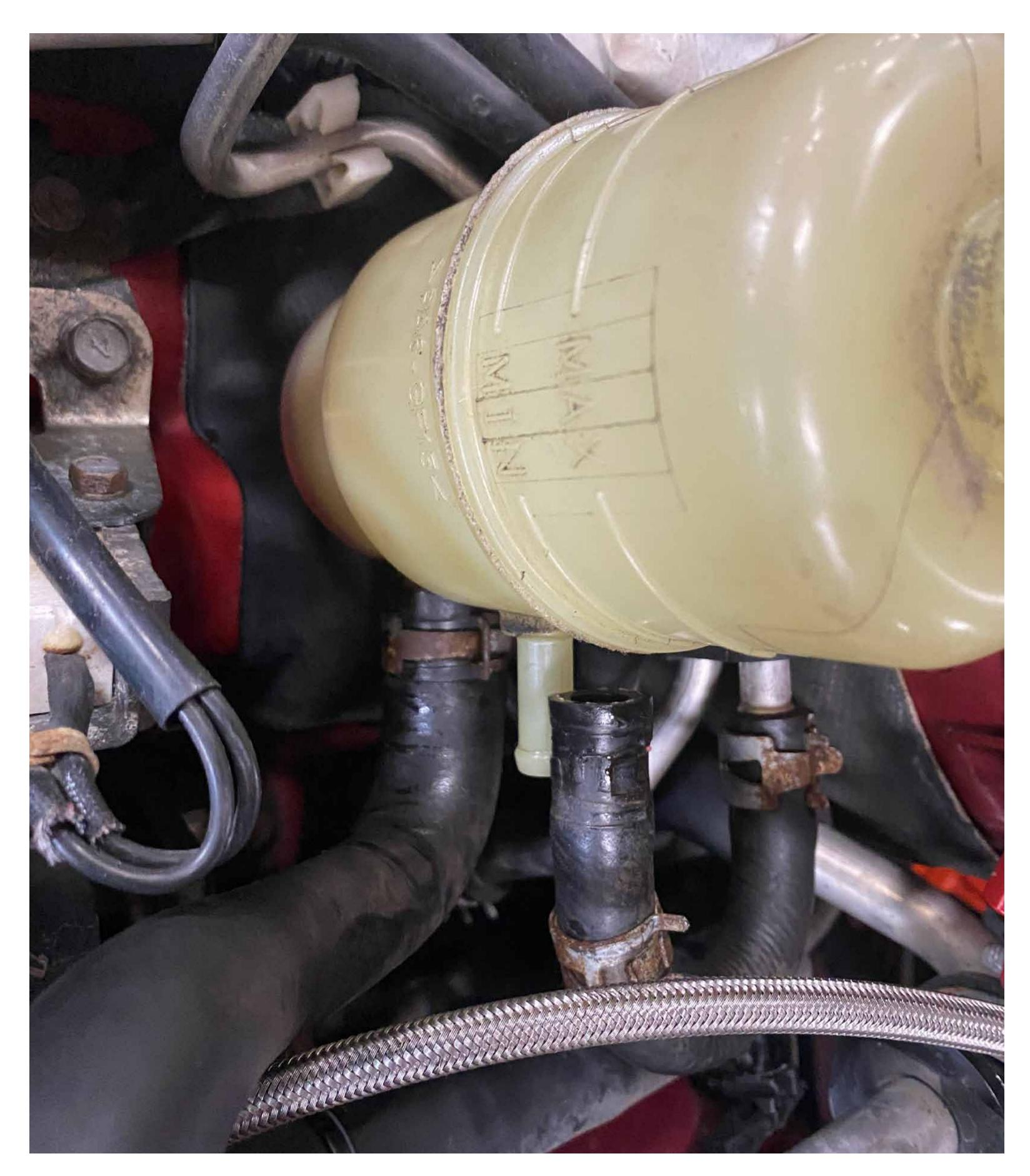
Remove upper power steering reservoir hose from the reservoir. If you own a fluid suction pump now would be the time to remove as much of the power steering fluid in the reservoir as possible
