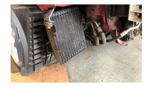
3. REMOVE BRACKET BOLTS HOLDING THE FACTORY OIL COOLER TO THE VEHICLE
