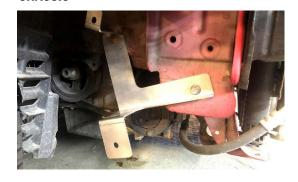
8. REUSE THE RUBBER GROMMETS FROM YOUR OLD OIL COOLER (OR REPLACE), INSTALL THEM INTO THE BRACKET AS SHOWN
