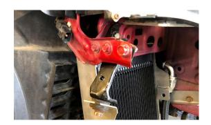
10. MEASURE YOUR FACTORY OIL COOLER LINES FOR REFERENCE, AND INSTALL THE BANJO TO -10 FITTINGS ON THE BLOCK. NOW ASSEMBLE ONE OF THE 90\* FITTINGS ON THE END OF THE HOSE, ROUTE THAT HOSE AS IT WILL RUN TO VERIFY LENGTH TO THE COOLER. CUT AND ASSEMBLE LINE, AND REPEAT FOR SECOND LINE. NOTE, THE DRIVERS SIDE PORT WILL USE THE STRAIGHT FITTING ON THE BLOCK.
