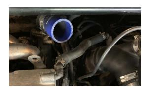
5. REMOVE VALVE COVER BARB, USE A VICE GRIP OR CHANNEL LOCKS TO SLOWLY WIGGLE AND PULL THE FITTING OUT OF THE VALVE COVER, USE HEAT IF NEEDED
