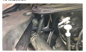
14A-B. REMOVE CAP FOR THE OVERFLOW AND THE OVERFLOW LEVEL INDICATOR, FILL UNTIL BOBBER REACHES HALF FULL, REINSTALL CAP
