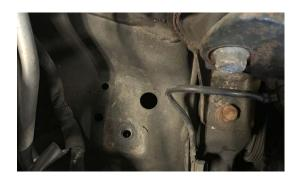
11. INSTALL MAP CATCH CAN INTO PLACE, SECURING WITH THE FACTORY BOLT HOLE USED FOR THE FACTORY OVERFLOW. THE KIT INCLUDES A NYLOC NUT THAT SECURES UNDERNEATH TO PREVENT THE BOLT FROM COMING LOOSE DURING HEAVILY SPIRITED DRIVING OR LARGE AMOUNTS OF VIBRATIONS.
