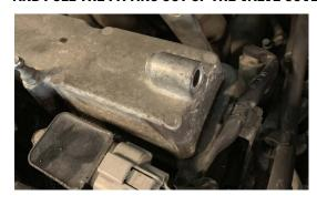
6. REMOVE VALVE COVER FITTING BY UNTHREADING IT WITH A 23MM SOCKET
