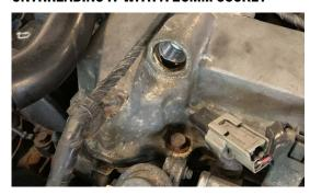
7. INSTALL INCLUDED - 10AN FITTING INTO VALVE COVER BY THREADING IT IN WITH A 23MM SOCKET, MAKE SURE TO TIGHTEN ALL THE WAY DOWN SEATING O-RING.
