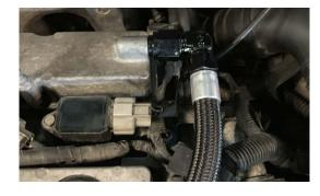
13A-B. RUN RUBBER COOLANT OVERFLOW LINE TO RADIATOR
