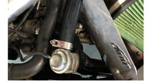
13.TRIM FACTORY LOWER TUBE FOR THE RECIRCULATION VALVE TO 3.25" LENGTH
