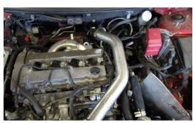
2. REMOVE TWO TURBO TO MANIFOLD NUTS, AND TWO STUDS
