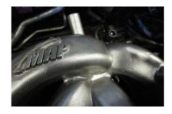
7. UTILIZING THE INCLUDED BOLTS, THREAD THEM INTO THE UPPER RIGHT, AND UPPER LEFT CORNERS OF THE MANIFOLD AND BEGIN TO SNUG THEM UP. REINSTALL THE OTHER EIGHT MANIFOLD TO HEAD NUTS AND TIGHTEN THEM ALL
