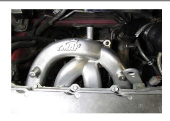
6. INSTALL THE OTHER THREE BOLTS - ONE STOCK, 2 INCLUDED - INTO THE MANIFOLD. THE LONGER OF THE TWO INCLUDED ONES GOES INTO THE DRIVERS UPPER BOLT HOLE.
