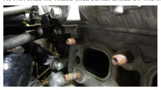
5. REINSTALL THE GASKET, AND SLIDE THE NEW MANIFOLD BACK IN THE SAME WAY THE STOCK ONE WAS REMOVED, BY TILTING AND SLIDING FROM THE REAR OF THE ENGINE BAY. MAKE SURE TURBO GASKET IS ON THE HOUSING AND INSTALL THE LOWER/INNER DRIVERS SIDE BOLT FROM THE MANIFOLD TO THE TURBO FIRST, AND SNUG THE BOLT DOWN, AS OTHERWISE YOU WILL NOT BE ABLE TO GET TO IT IN THE CAR EASILY WITH ALL OTHER BOLTS IN, ONCE THREADED IN,
