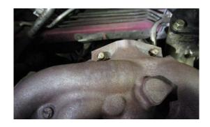
3. REMOVE TEN MANIFOLD TO HEAD NUTS.
