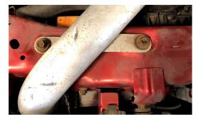
4. REMOVE FACTORY COUPLERS FROM INTERCOOLER AND REAR UPPER COOLER PIPE AND RE-PLACE THEM WITH THE COUPLERS INCLUDED IN KIT
