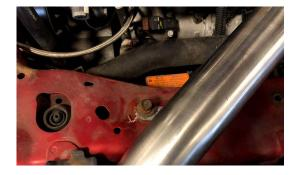
7. POSITION THE NEW FRONT UPPER PIPE TO YOUR DESIRED FITMENT, THEN START BY TIGHTENING THE MOUNTING TAB BOLT AND THEN TIGHTEN THE T-BOLT CLAMPS, START CAR AND CHECK FOR LEAKS.
