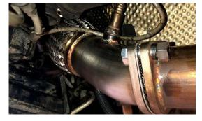
**6. PLACE TAPE ON DOWNPIPE TO HOLD GASKET DOWNPIPE IN PLACE - START THREADS ON ALL BOLTS**
