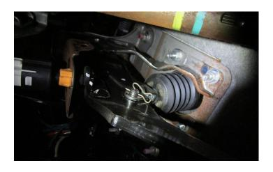
13. REMOVE COTTER PIN AND PIN FROM THE BRAKE PEDAL AND MASTER CYLINDER CLEVIS, AND THE FOUR NUTS AROUND THE PEDAL HOLING IN THE BOOSTER.
