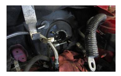
14. REMOVE LEVEL SENSOR CONNECTOR AND THE TWO NUTS HOLDING THE MASTER TO THE BOOSTER, PULL MASTER, AND THEN BOOSTER FROM THE CAR.
