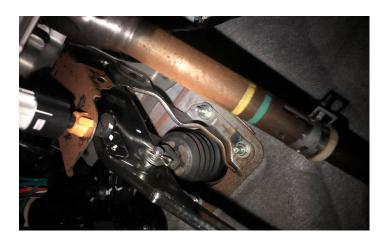
22. INSTALL THE MASTER BACK ONTO THE BOOSTER, ATTACH FEED LINE TO CLUTCH MASTER AND BRAKE LINES TO MASTER, THEN PLUG IN LEVEL SENSOR.
