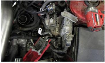
7. UNBOLT ECU BRACKET, AND PULL ASSEMBLY TO THE SIDE 8A-B. REMOVE BRACKET TRAY, 3 BOLTS WILL HOLD IT IN, SET WHILE STILL CONNECTED.
