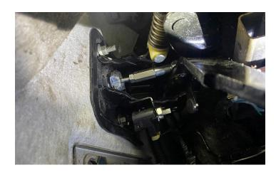
21. SLIDE BOOSTER BACK INTO CAR, REINSTALL THE 4 NUTS, AND THE REMOVED PIN AND COTTER PIN.
