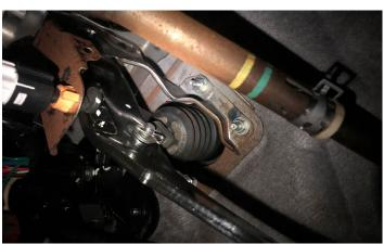
26. INSTALL THE MASTER BACK ONTO THE BOOSTER, ATTACH FEED LINE TO CLUTCH MASTER AND BRAKE LINES TO MASTER, THEN PLUG IN LEVEL SENSOR.
