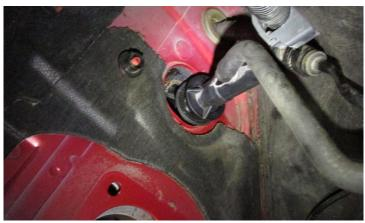
17A-B. REMOVE MODULE FROM LEFT OF CLUTCH PEDAL TO GAIN ACCESS TO FIREWALL.
