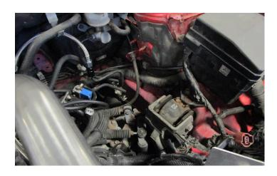
9. REMOVE CLUTCH LINE RETAINING CLIP, TAP WITH A FLATHEAD SCREWDRIVER AND A MALLET TO UNSEIZE THE CLIP, REMOVE WITH A PLIERS OR CHANNEL LOCKS.
