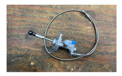
22. FOR THIS STEP, A SECOND SET OF HANDS WILL MAKE IT MUCH EASIER. INSTALL THE MASTER AND MOUNTING PLATE TO THE FIREWALL, YOU WILL USE THE TWO LONGER M 10 BOLTS, AND 2 M 10 FLANGE NUTS TO ASSEMBLE. TIGHTEN ONCE INSTALLED.
