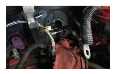
15. REMOVE CLEVIS ON CLUTCH MASTER CYLINDER TO CLUTCH PED-AL, A FLATHEAD SCREWDRIVER AND LIGHT FORCE WILL POP IT OFF.
