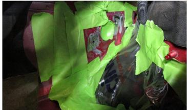
20A-D. AFTER GRINDING, WE RECOMMEND PRIMING AND PAINTING THE AREA TO PREVENT ANY CORROSION IN THE FUTURE. LET DRY.
