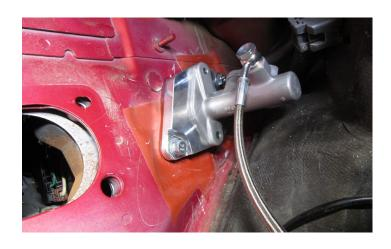
23. WITH THE PEDAL ALL THE WAY OUT, SLIP THE BALL END OF THE ADAPTER CLEVIS OVER THE BALL ON THE PEDAL. MAY NEED TO WIGGLE THE ADAPTER TO GET IT ALL TO SEAT RIGHT. SECONDARY LOCKING PIN NOT NEEDED
