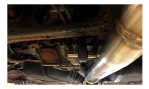
8. INSTALL INCLUDED V BAND CLAMP, ENSURE YOU HAVE THE PROPER FITMENT BEFORE TIGHTENING
