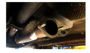
6. INSTALL FRONT HALF OF THE CAT BACK ONTO THE CATALYTIC CONVERTER OR TEST PIPE
