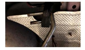
4. REMOVE THE RUBBER HANGER NEAR THE DIFF, THIS SHOULD ALLOW THE FACTORY CATBACK TO BE COMPLETELY REMOVED
