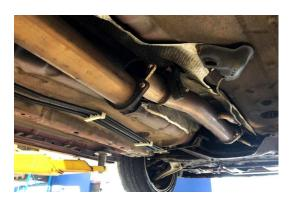
3. REMOVE THE 2 RUBBER HANGERS SECURING THE MUFFLER TO VEHICLE
