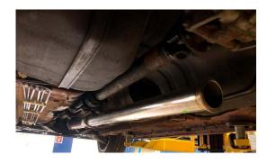
7. INSTALL RUBBER HANGERS ONTO THE MUFFLER SECTION, THEN INSTALL THE MUFFLER INTO THE VEHICLE SECURING IT BY THE RUBBER HANGERS
