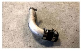
13. SLIDE MAP INTERCOOLER INTO THE LOW-Er charge pipe, then back into place
