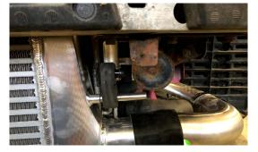
14. RE SECURE INTERCOOLER ONTO RUBBER HANGERS, BE SURE TO Install the hanger bracket you removed back into place
