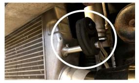
12. INSTALL INCLUDED COUPLERS AND CLAMPS ONTO LOWER CHARGE PIPE
