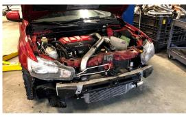
6. LOOSEN THE 4 CLAMPS HOLDING THE COUPLERS ONTO THE UPPER CHARGE PIPE, THEN REMOVE THE 2 BOLTS HOLDING THE CHARGE PIPE TO THE CORE SUPPORT
