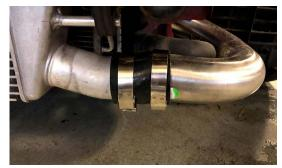
9. REMOVE BOTTOM BRACKET BOLTS, REMOVE RUBBER Hanger from intercooler on passenger side
