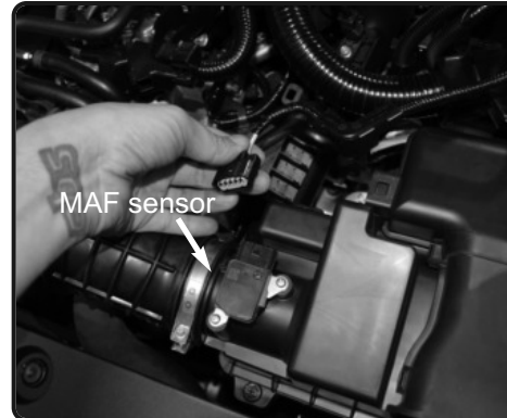
3. Disconnect the MAF sensor.
