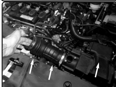
6. Pull back the intake tube from turbo housing.
