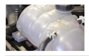
21. INSTALL THE LOWER COUPLER TO INTER-COOLER WITH CLAMP, AND THE THROTTLE BODY
