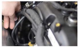
26. ON THE BACK OF THE INTAKE MANIFOLD WILL BE A WHITE CLIP WITH A VACUUM LINE COMING OUT OF IT, CUT THE LINE  $\sim$  3-4" AWAY FROM THE CLIP AND INSTALL THE
