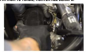
24. REINSTALL INTAKE - REMEMBER TO INSTALL THE BLOW OFF VALVE, AIT SENSOR, AND AIR FILTER
