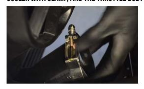
22. SLIDE THE DRIVER SIDE PIPE INTO PLACE AND TIGHTEN CLAMPS
