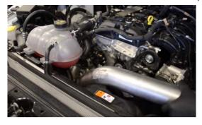
5. DETACH COOLANT RESERVOIR AND SECURE OUT OF THE WAY
