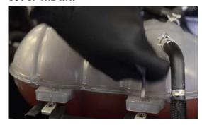
6. REMOVE THE TWO TOP MOUNTS SECURING THE RADIATOR TO THE CORE SUPPORT
