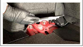
REMOVE LOWER END LINK BOLT WITH 14mm, LOWER STRUT BOLT WITH 17mm, AND OUTER CONTROL ARM BOLT WITH 17mm.
