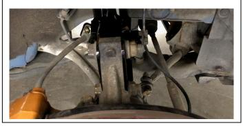
SECURE BRAKE LINE TO BRACKET USING SUPPLIED BOLT AND NUT. SECURE ABS LINE TO BRACKET USING OEM 12mm BOLT (STYLE 1) OR CLIP (STYLE 2)
