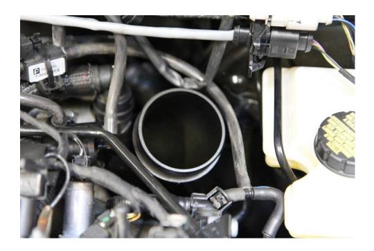
Remove the T30 screws holding the factory inlet pipe to the turbo. Bolt does not need to be removed.
