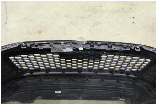
Step 17: Reinstall bumper, plug in foglights. Reinstall splash guard and fender liner.
