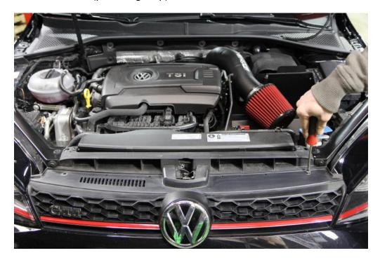
**Step 2:** Remove 3x fender liner screws on both sides of the car.
