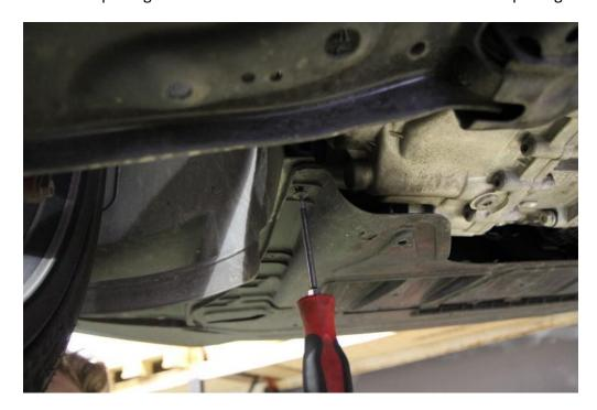
**Step 4:** Remove 7x screws under the bumper.
