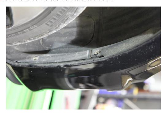
**Step 3:** Remove 8x splash guard screws from the bottom of the car. Remove splash guard.
