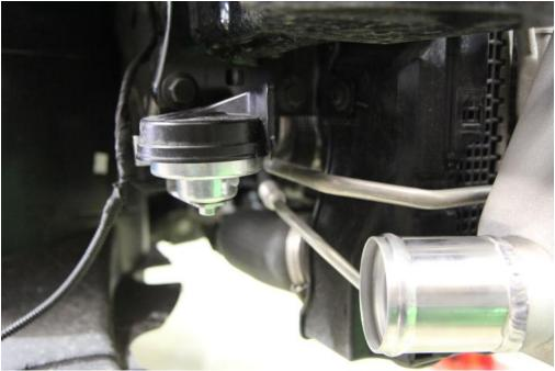
**Step 12: OPTIONAL**, this step applies only to cars with SAI system - remove the mounting bolt for SAI pump, loosen the second mounting bolt on the back. Install supplied bracket to move pump out of the way.
