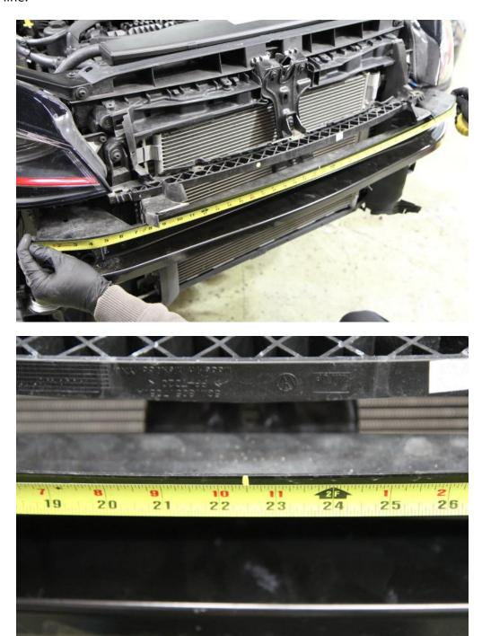
**Step 7:** Measure 11.75" from the middle of the right hole on intercooler mounting bracket and mark the center line.
