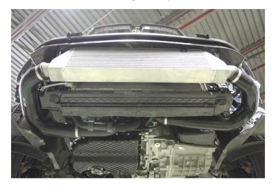
**Step 16:** Remove two plastic covers from the bumper as shown.
