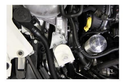
Step 6: Install hoses and secure them using crescent wrench. Install hose separator, tighten using ¼" allen. Reinstall coilpacks and attach harness.
