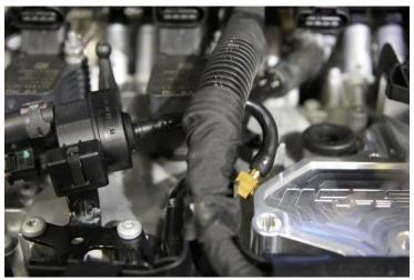
Step 5: Install catch can as shown, using M6x40mm and M6x16mm socket head screws. Attach the catch can to bracket using 2x M6x12mm button head screws. On Golf R and S3 models, you will have to install the supplied filler hose as shown. Secure hose away from moving components using supplied tie wraps. 13mm wrench can help to tighten the threaded post.
