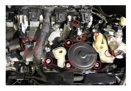
Step 2: Remove 7x T30 torx screws from factory breather plate and 1x T30 screw holding the rear PCV hose on. Remove the hose from N80 valve using pliers, take care not to break anything. See photo in step 1.
