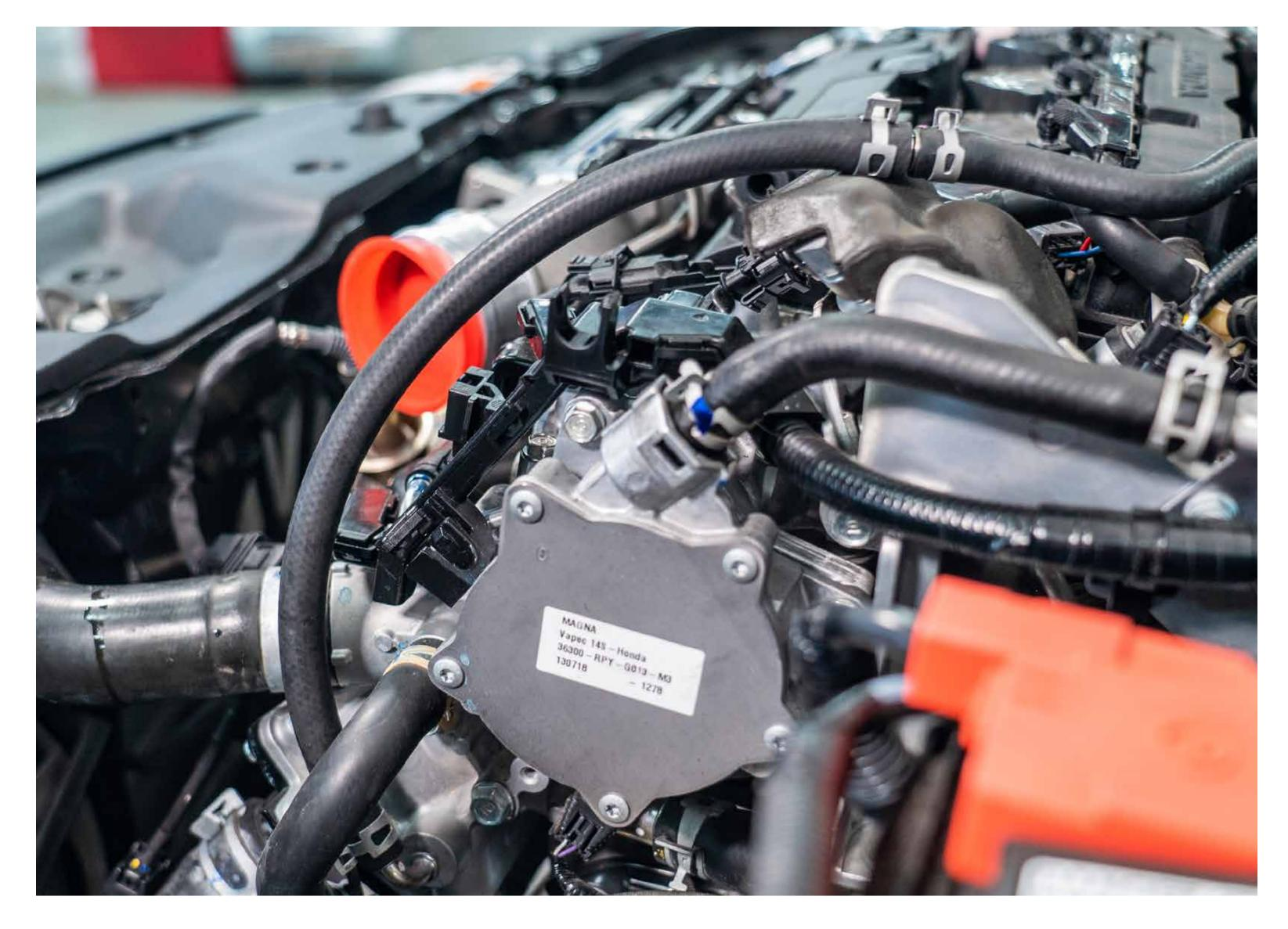
Install included coolant line with included barb and spring clamps
