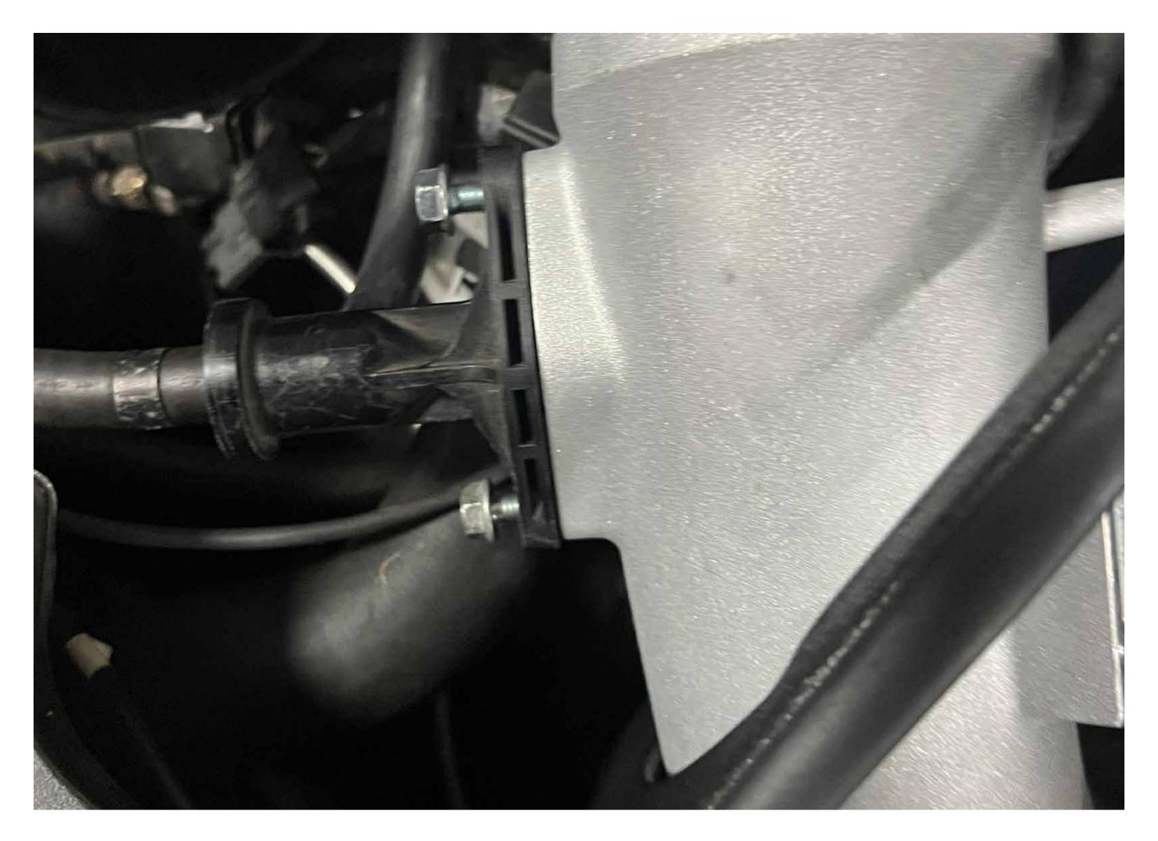
Before installing the intake tube into the coupler be sure to reinstall the venturi and its hoses onto the intake we have included extra hose to replace the existing hose as it may be too short, the hose from the charge pipe goes to the straight end of the venturi, the intake manifold hose goes to the 90 end of the venturi.
