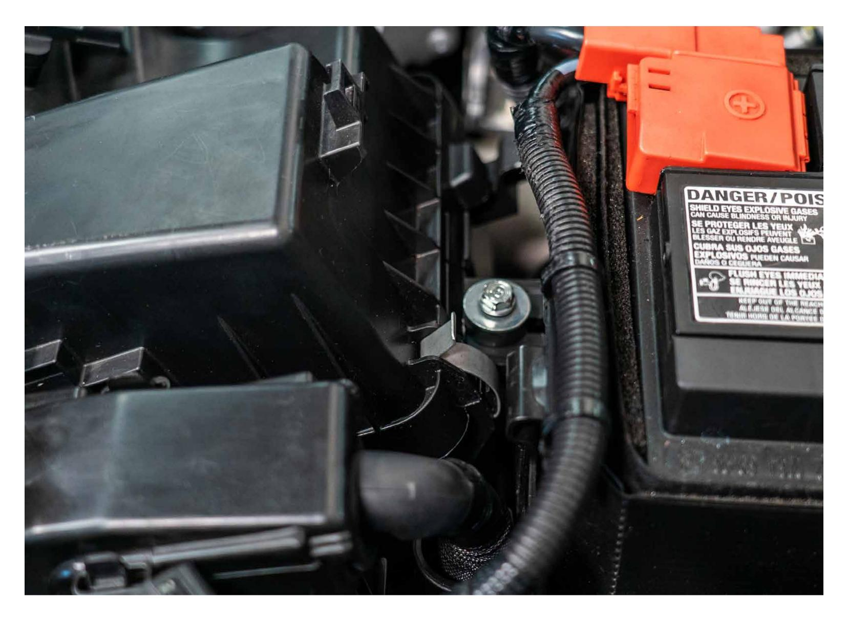
Remove locking tabs securing top half of the factory intake box to the lower portion
