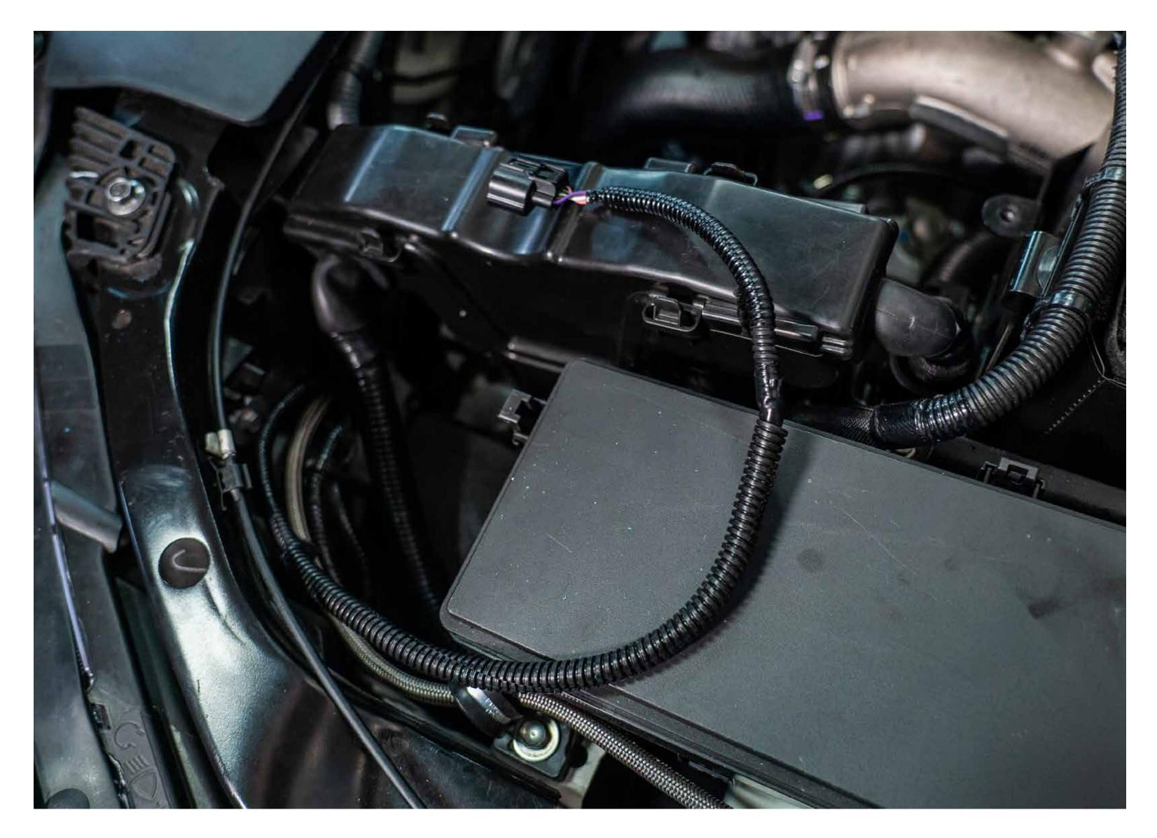
Remove factory MAF cover carefully with a small flathead screwdriver, then cover with included split tubing
