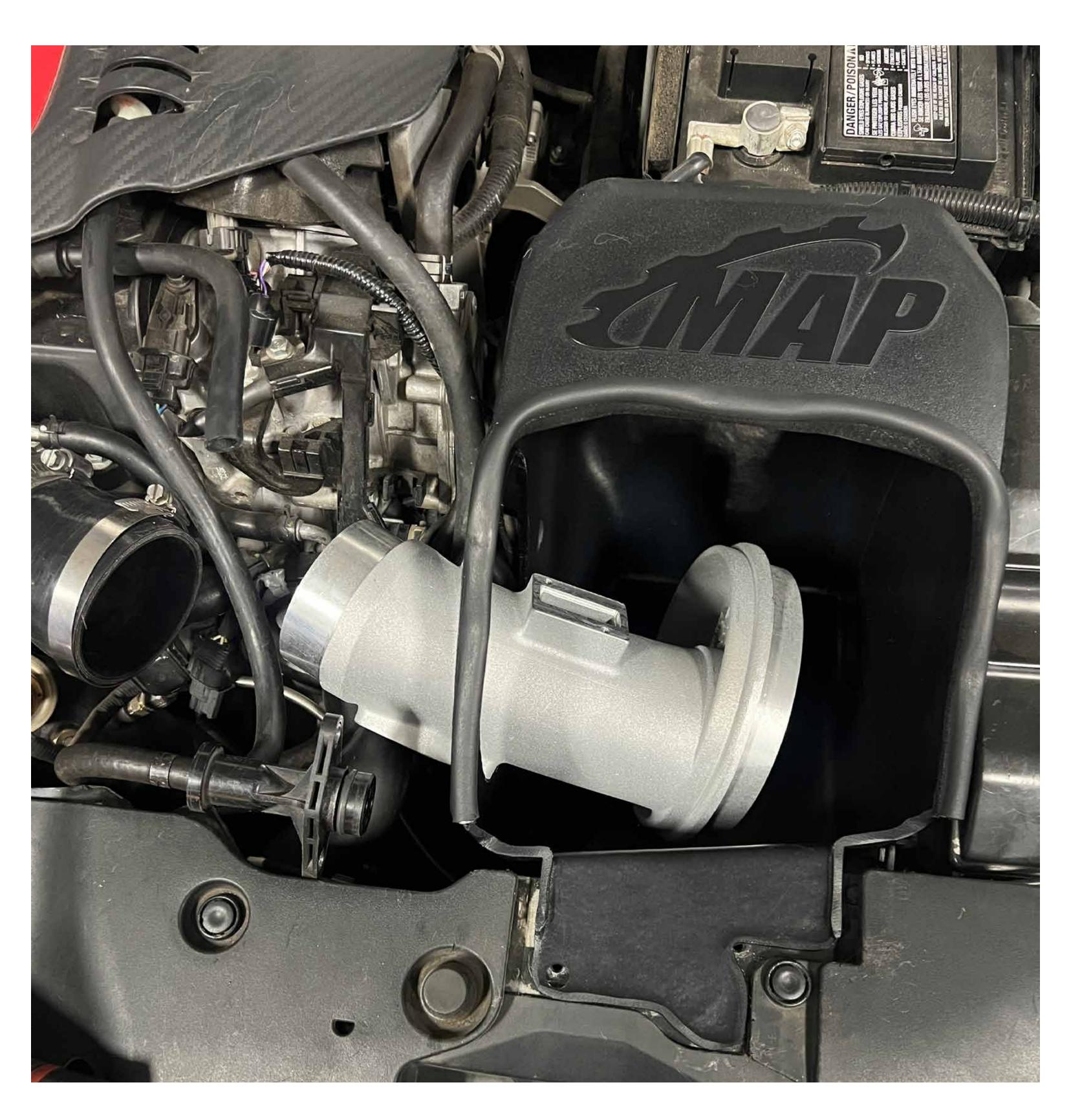
Side intake pipe through large opening in the air box housing
