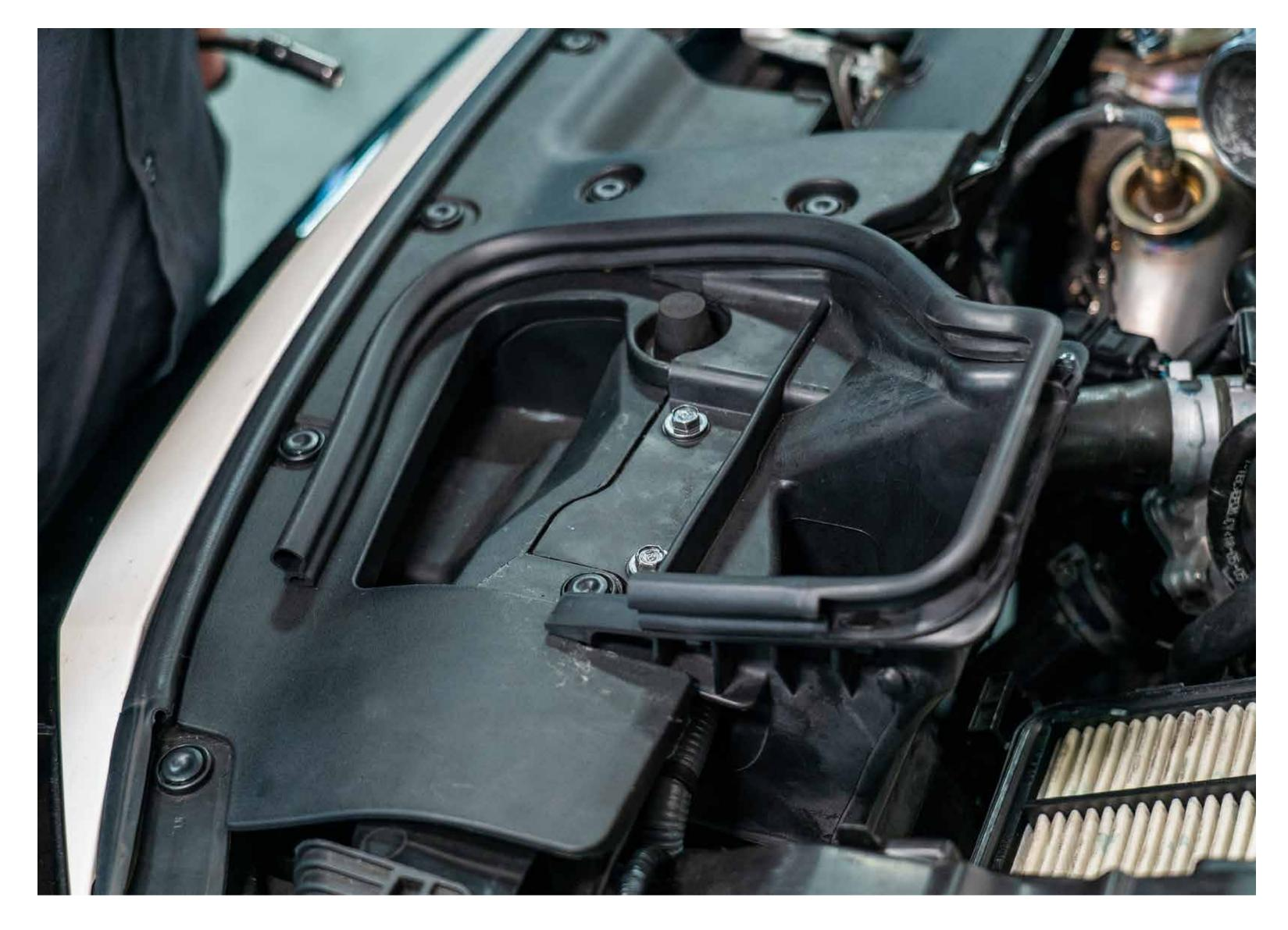
Remove intake inlet shroud bolts (10mm)
