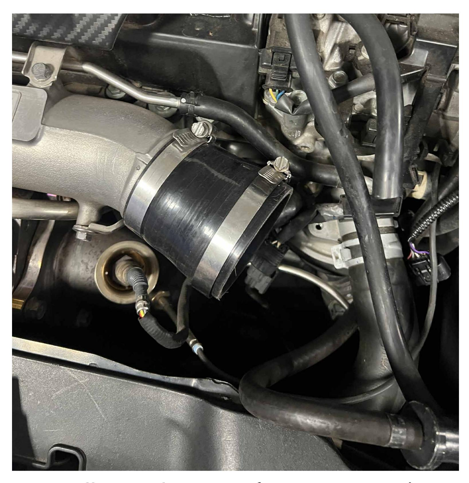
Install coupler onto factory overpipe and secure one side with clamp
