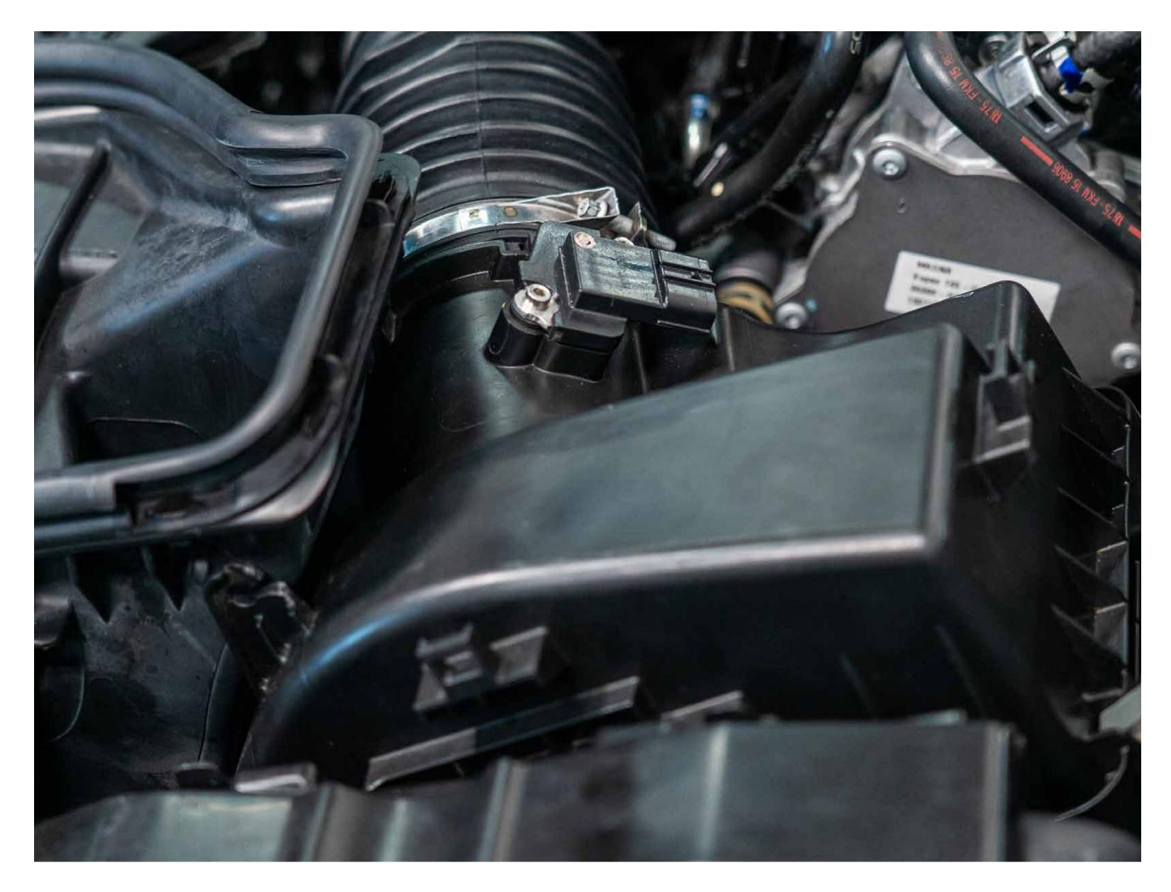
Start by disconnecting the MAF sensor connector
