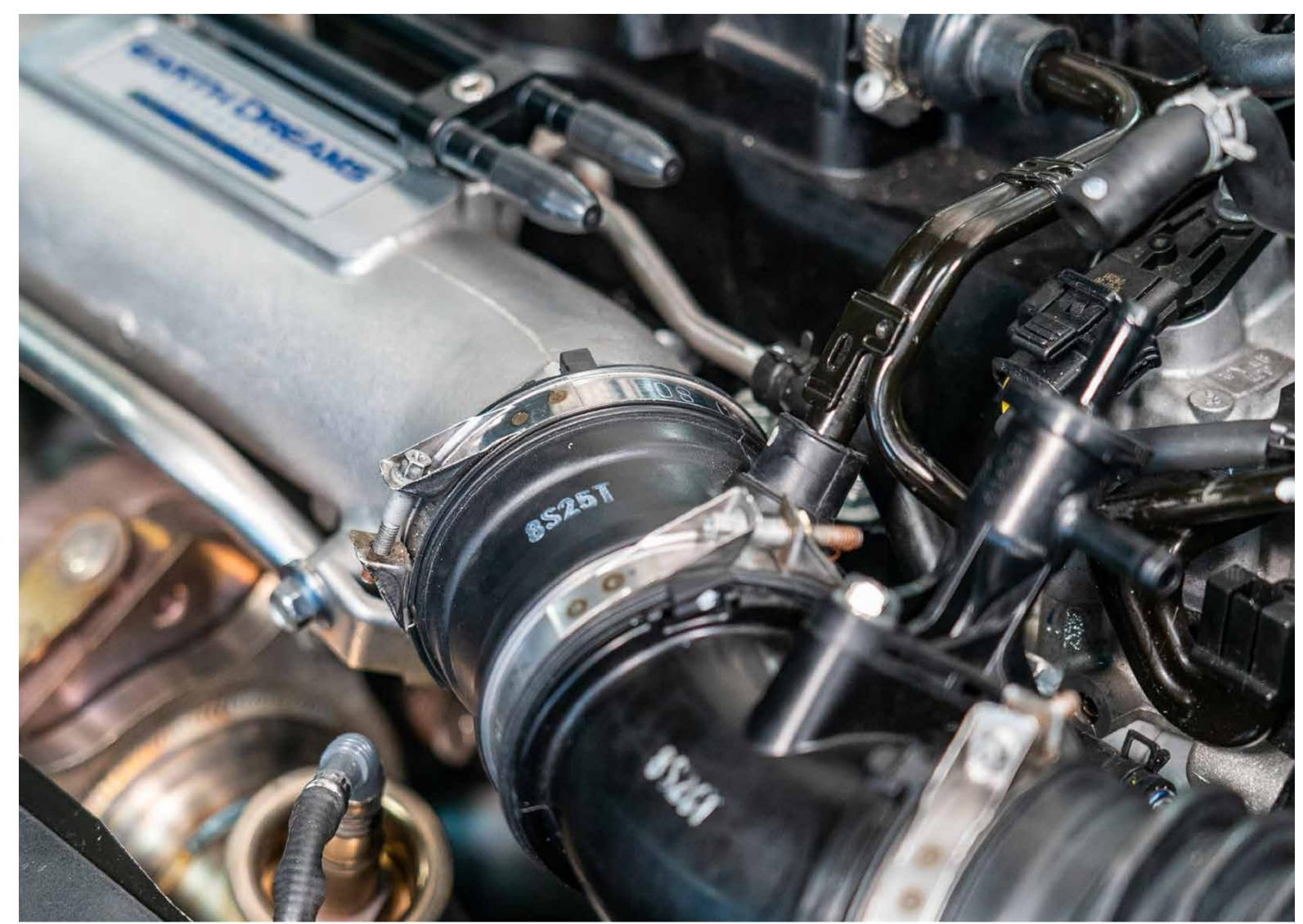
Remove clamp from valve cover-to-intake tube connection
