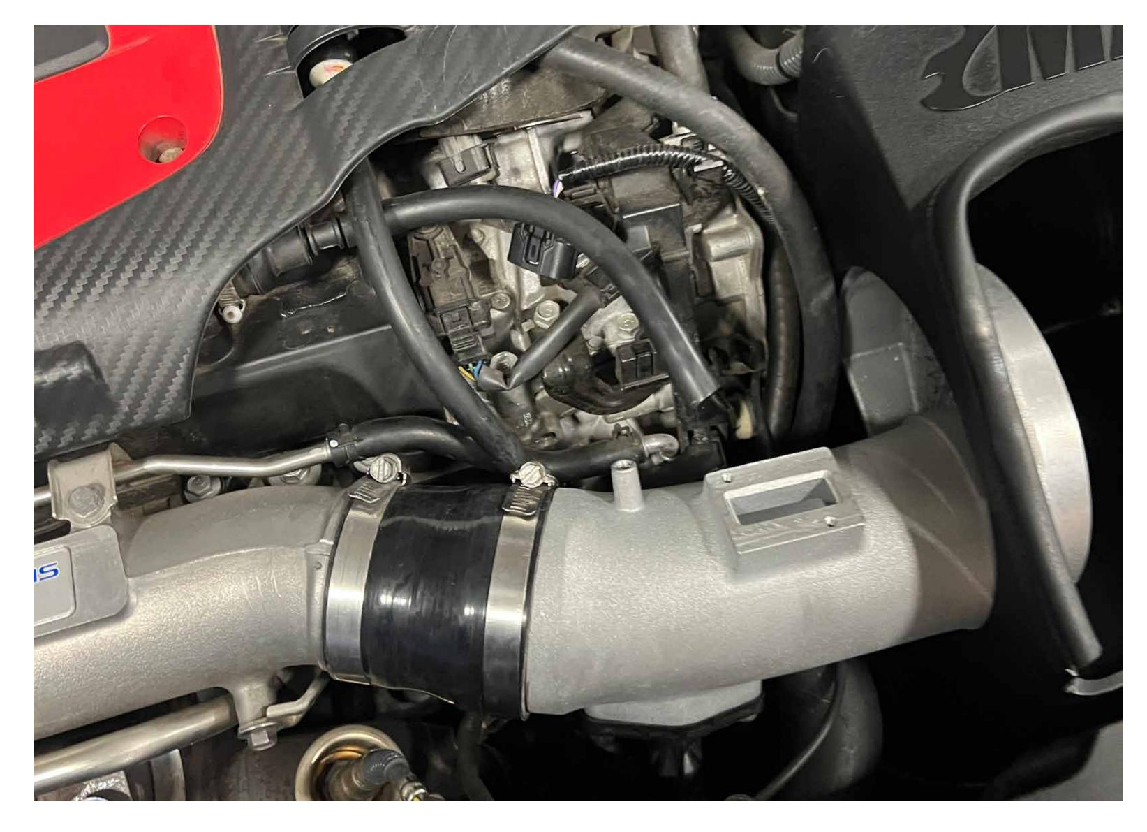
Install intake pipe into overpipe coupler and secure with clamps
