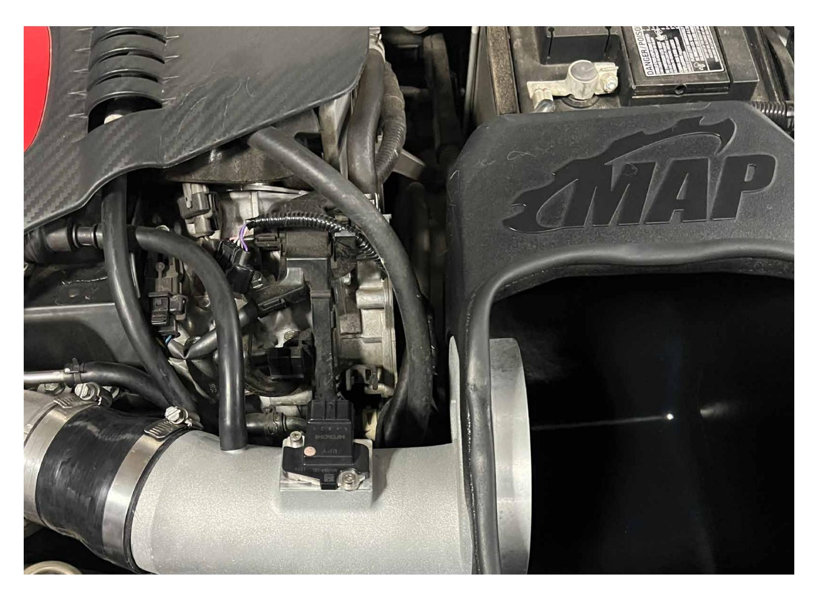
Install plastic union onto the included hose, this will install into the valve cover and connect to the intake tube
