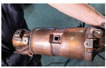
15. INSTALL THE POST CAT 02 SENSOR INTO THE MAP DOWNPIPE
