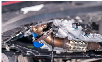
11. REMOVE 3 14MM NUTS ON THE DOWNPIPE TO FRONT PIPE CONNECTION
