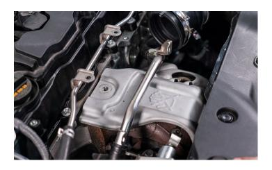
7. AT THIS POINT, YOU WILL BE ABLE TO REMOVE THE BOLTS HOLDING THE FACTORY HEAT SHIELD ON. IT WILL TAKE SOME MANEUVERING OF COOLANT CROSSOVER PIPES BUT YOU WILL BE ABLE TO SLIDE THE HEAT SHIELD UP AND OUT
