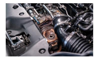
8. REMOVE THE 4 14MM BOLTS AND NUTS CONNECTING THE FACTORY DOWNPIPE TO THE TURBO OUTLET
