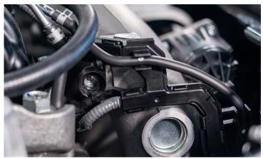
4. REMOVE 2 BOLTS (12MM) HOLDING THE INLET PIPE ONTO THE TURBO INLET
