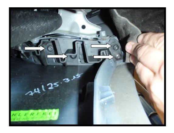
5. Remove the T30 torx from the back of the light. This is hard to see and reach but you can access from the inner arch.
