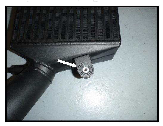
18. Attach the air temperature sensor to the bracket supplied in the kit.
