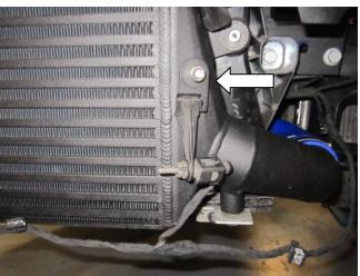
22. Fit the ACC module to the new bracket provided. This can now be fitted to the crash bar, and reconnected to the wiring loom.
