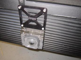
23. For facelift models ie DAZA engine code a different ACC module is used please remove the oem bracket as pictured below and mount using the OEM fasterners and m6 flange nuts provided.
