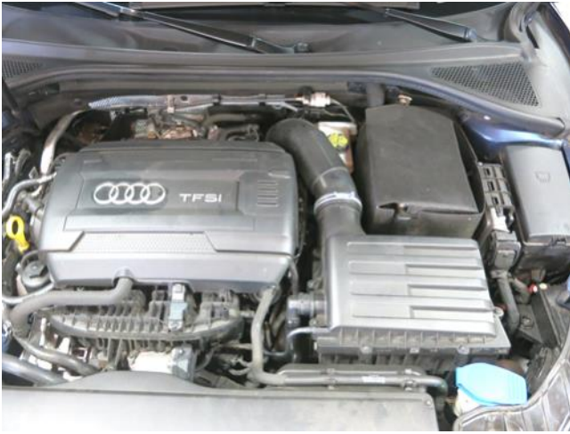
STOCK INTAKE INSTALLED
