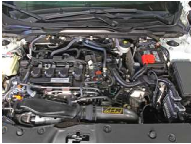
AEM INTAKE INSTALLED
