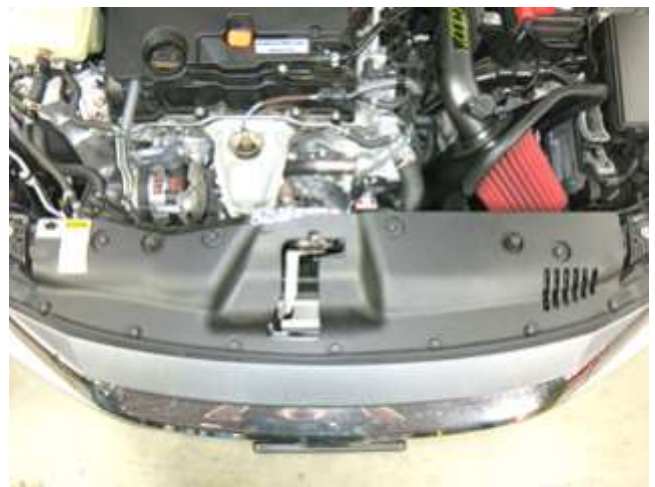
p. Re-install the front shroud cover on to the vehicle with the nine push-in clips removed in step 2a.
