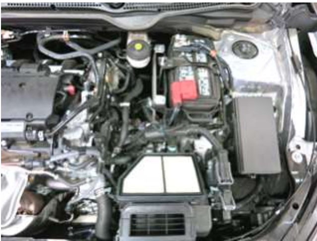
g. Remove the upper air box with the intake arm.
