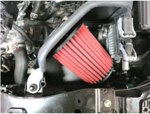
k. Lower the AEM filter with hose clamp into the AEM heat shield as shown.
