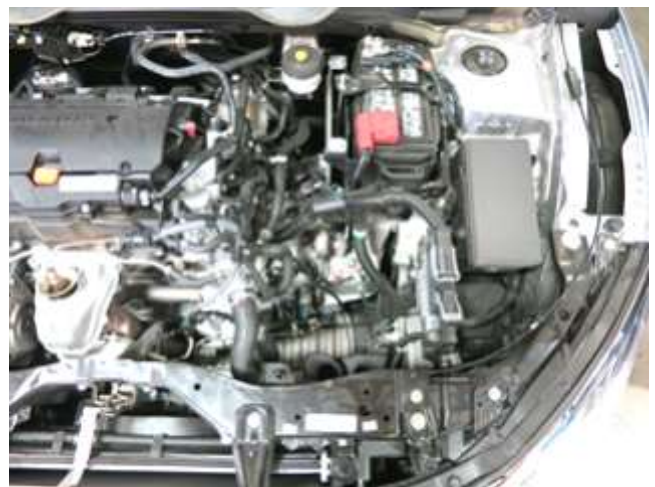
j. Lower air box removed.
