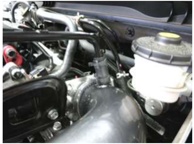
l. Align the previously installed hose on the AEM intake to the factory vent hard line and secure with the spring clamp.
