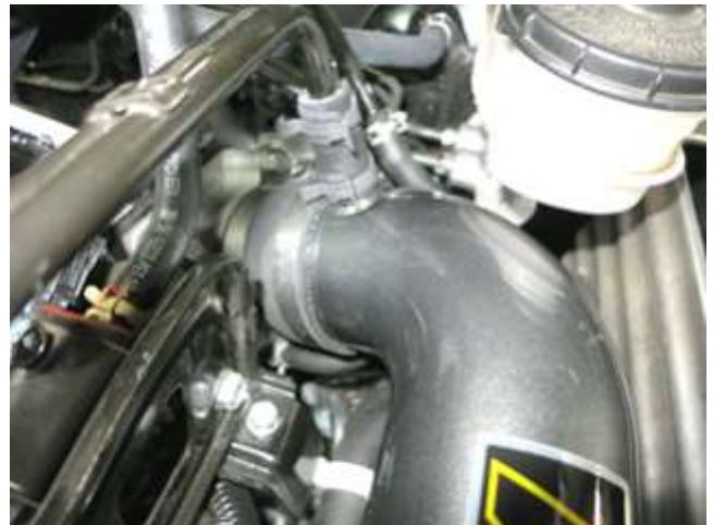
n. Connect the other end of the AEM intake tube into the coupler that was installed on the throttle body.
