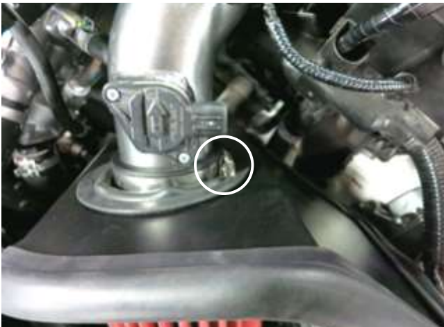
m. Connect the AEM intake tube to the AEM filter, and tighten the hose clamp (30 in. lb.) to secure the filter to the tube. Connect the MAF sensor connector.
