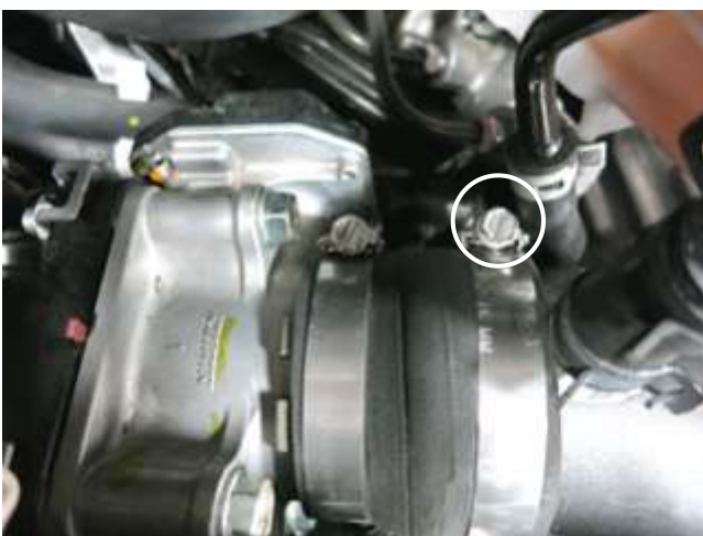
o. Once the AEM intake tube is properly aligned with the coupler and the heat shield, tighten the circled hose clamp (30 in. lb.).
