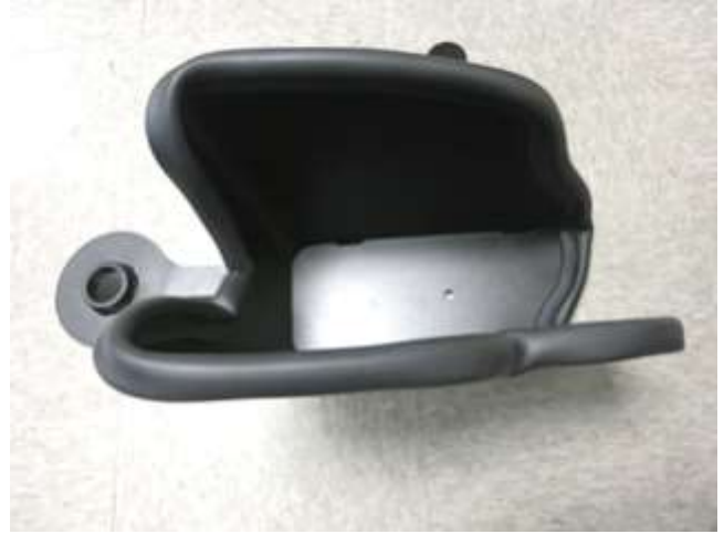
b. Install the supplied rubber edge trim onto the AEM heat shield assembly as shown.
