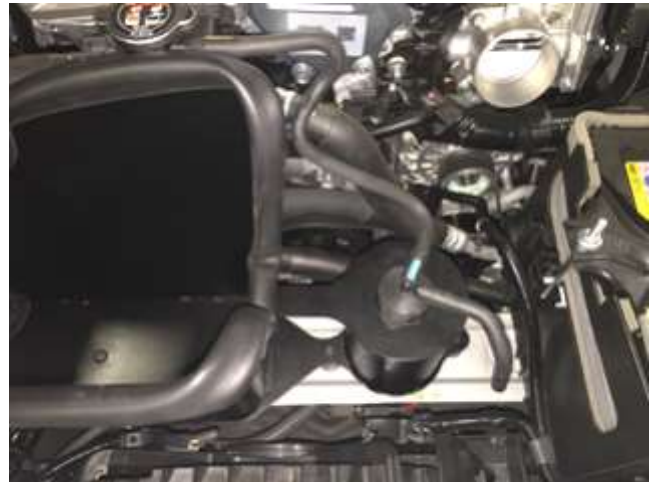
d. Transfer the coolant from the factory tank into the AEM reservoir and seal with factory cap. The capacity of the AEM reservoir is different from the factory reservoir but it does not affect the functionality.
