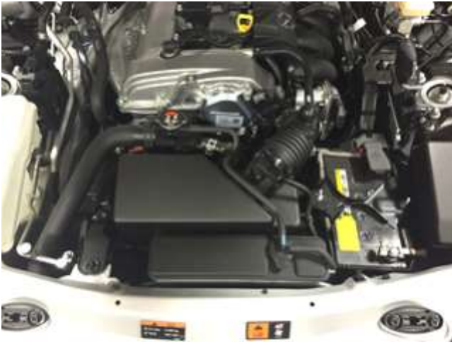
STOCK INTAKE INSTALLED
