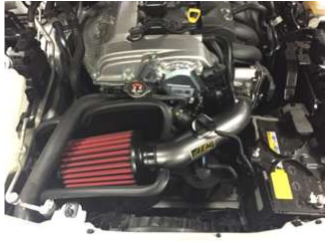
AEM INTAKE INSTALLED
