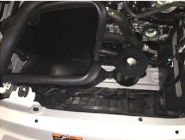
c. Install the complete heat shield assembly into the engine compartment as shown and secure with supplied hardware.
