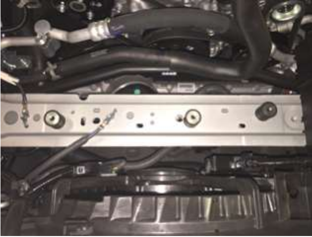
a. Install the supplied rubber isolator mounts into the engine compartment as shown.
