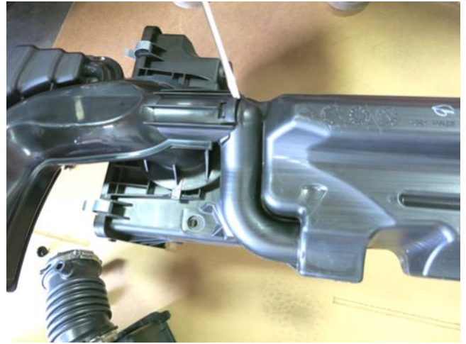
b. Unclip the resonator chamber from the cold air scoop while rotating the cold air scoop gently.
