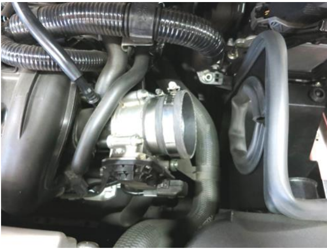
i. Install provided coupler with hose clamps onto throttle body. Do not tighten hose clamps at this point.
