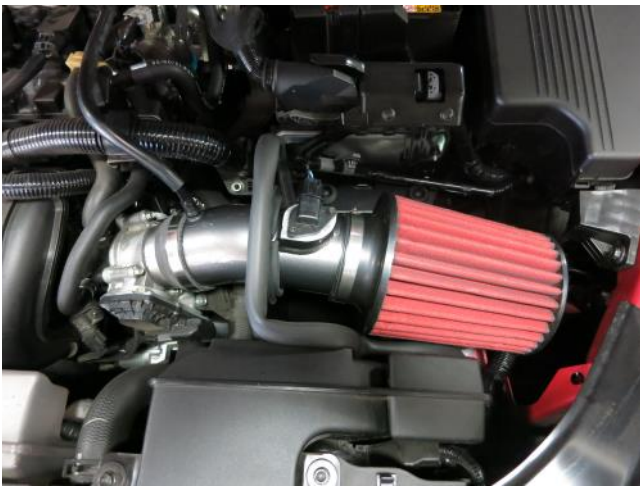
m. Check for clearance around the filter, heat shield and intake tube then tighten all hose clamps. Reinstall the engine cover.
