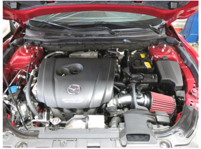
p. Finished installation of AEM Intake System.
