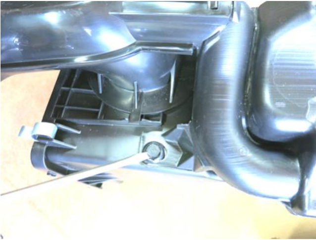
a. Unclip the two plastic retainers securing the cold air inlet scoop to the factory air box.
