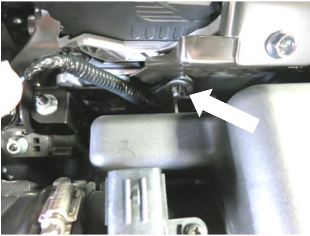
e. Use needle nose pliers to unclip wire harness from air box.
