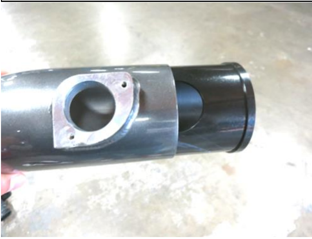
g. Install the supplied MAF sleeve into the AEM intake tube and line up the opening to the MAF
