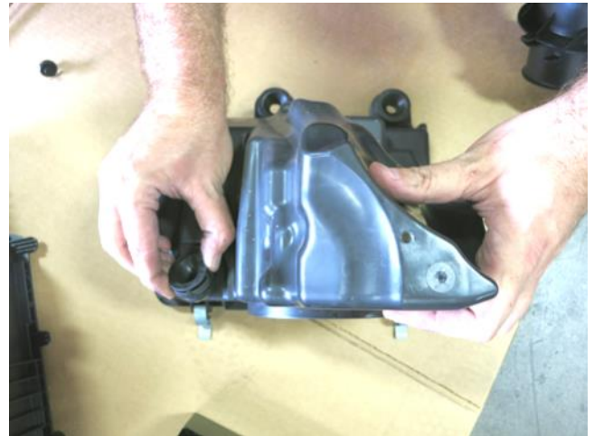
d. Remove the three rubber grommets from the factory air box and insert them into the AEM heat
