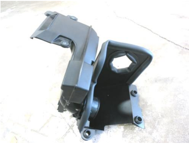
e. Install edge trim around the intake tube pass through hole and around the AEM heat shield then install the air scoop into the AEM heat shield assem-
