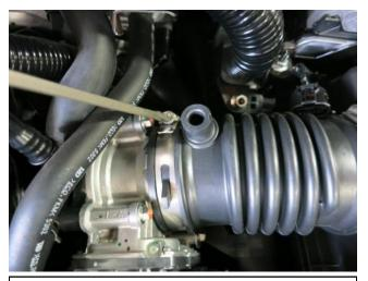
d. Loosen hose clamp securing coupler to throttle body.
