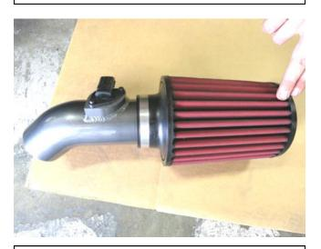
j. Loosely install the AEM air filter onto the intake tube.
