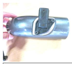
h. Install MAF sensor into the AEM intake tube using provided hardware.
