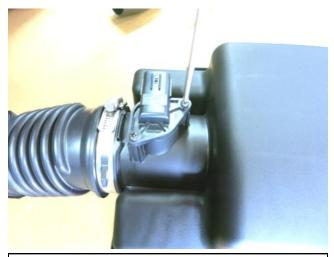
g. Remove MAF sensor from the factory air box using a small Philips head screw driver.
