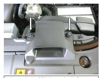
h. Loosen the two M6 bolts securing the factory cold air inlet scoop.
