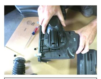
c. Rotate the cold air scoop until it will separate from the lower air box.
