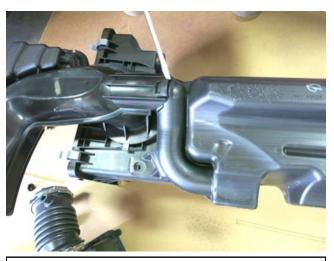
b. Unclip the resonator chamber from the cold air scoop while rotating the cold air scoop gently.
