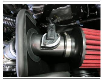
m. Connect the MAF sensor harness to the sensor and tighten all of the hose clamps.
