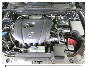
p. Finished installation of AEM Intake System.
