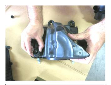
d. Remove the three rubber grommets from the factory air box and insert them into the AEM heat shield.
