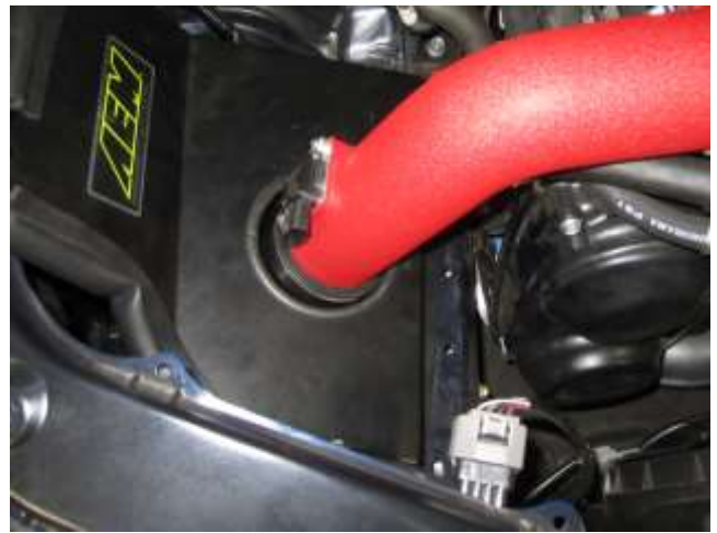
h. Install the filter, heat shield, and tube assembly into the vehicle.
