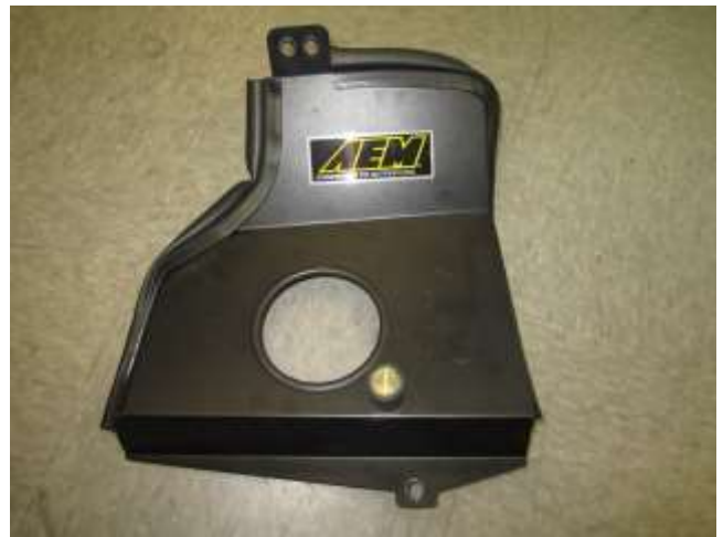
f. Completed heat shield assembly.
