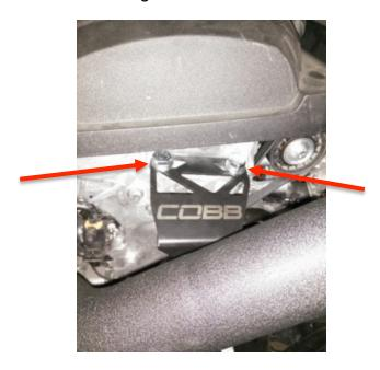
9. Now you can move the Intake Pipe to where you are able to loosely fasten the pipe to the bracket using an M8 x 12 Flange Head Bolt along with the 8mm flat washer. Before doing so, make sure the intake pipe is fitted inside the cutout on the airbox. Use a 12mm socket to tighten.
