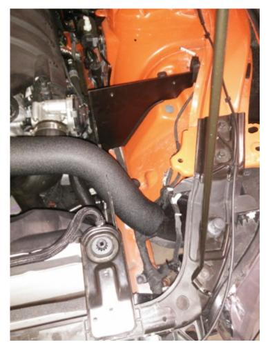
6. Using the M6 flange head bolt and the 6mm nylon washer, bolt down your new airbox using a 10mm socket in the same location using the mounting slot on the COBB Airbox. Tighten both bolts used to install the airbox.
