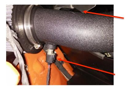
13. Now that the filter is in place and the sensors are connected, place the Airbox Lid on top of the airbox and fasten to the body of the airbox using the (4) SS Button Head M4 x 10 Screws and the (4) 4mm Black Nylon Washers. Use a 3mm Allen Wrench to tighten the screws.
