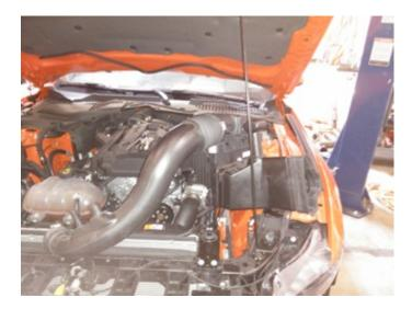
5. Remove remaining stock silicone hoses and the grommet used to hold the stock intake in place.
