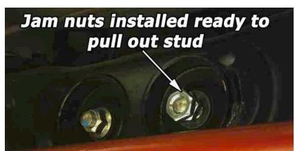
Shows nut removed, and jam nuts installed ready to remove stud from diff cover.
