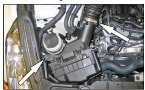
4. Loosen the hose clamp which secures the passenger side intake hose to the air box. Remove the bolt which secures the air box to the inner fender.
