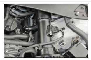
27. Reconnect the mass air sensor electrical connection.
