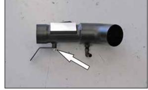
36. Install the tube mounting bracket onto the passenger side K&N® intake tube as shown and secure with the provided hardware.
