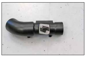
35. Install the mass air sensor into the passenger side K&N® intake tube and secure with the provided hardware.
