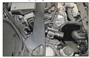
37. Install the K&N® intake tube into the coupling hose at the throttle body and align the bracket with the mounting hole in the heat shield. Adjust the tube and heat shield for proper fit and then secure with the provided hardware and hose clamp.
