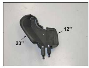
17. Install the trimmed edge trim onto the heat shield as shown.
