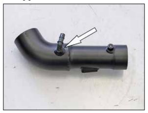
19. Install the provided 90° NPT vent fitting into the driver's side K&N® intake tube (27466) as shown. NOTE: Plastic NPT fittings are easy to cross thread. Install the vent fitting "hand" tight, then turn it two complete turns with a wrench.
