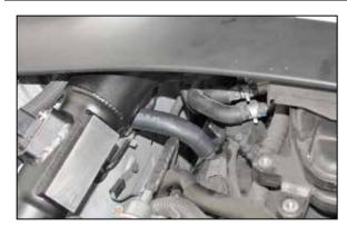
38. Install the 5" crank case vent hose onto the 90° fitting on the K&N® intake tube and then attach the open end to the vent port on the valve cover.
