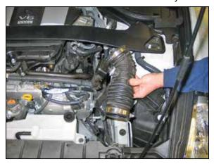
13. Remove the driver's side intake hose from the vehicle.
