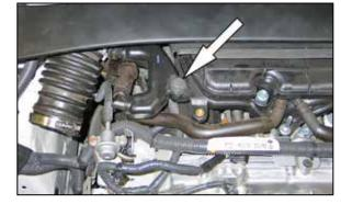
6. Remove the bolt shown which secures the crank case vent tube assembly to the intake plenum.
