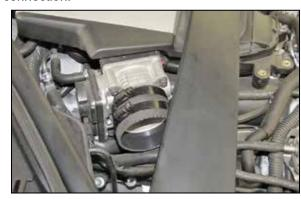
28. Install the coupling hose (084036) onto the passenger side throttle body and secure with the provided hose clamp.
