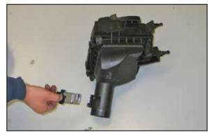
34. Remove the two screws securing the mass air sensor to the air box and then remove the mass air sensor from the air box.
