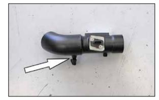
33. Install the provided 90° NPT vent fitting into the  $K\&N^{\otimes}$  intake tube (27642) as shown.
