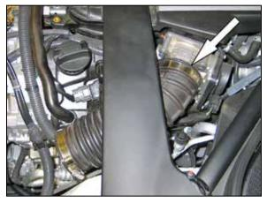
12. Loosen the hose clamp that secures the driver's side intake tube to the throttle body.
