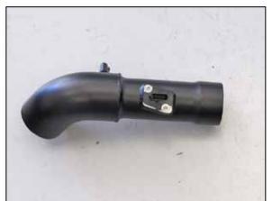
21. Install the mass air sensor into the driver's side  $K\&N^{\circledcirc}$  intake tube and secure with the provided hardware.
