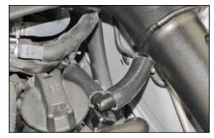
25. Connect the end of the crank case vent hose with the hose clamp to the 90° vent fitting on the driver's side K&N® intake tube and then connect the other end to the vent port on the valve cover. NOTE: Some trimming of the crank case vent hose may be necessary.
