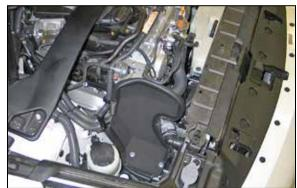
32. Install the heat shield assembly into the vehicle so that the mounting pins engage into the air box mounting grommets.
