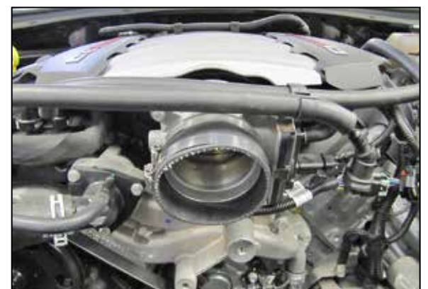
21. Install the provided coupler hose (08761) onto the throttle body and secure with the provided hose clamp.
