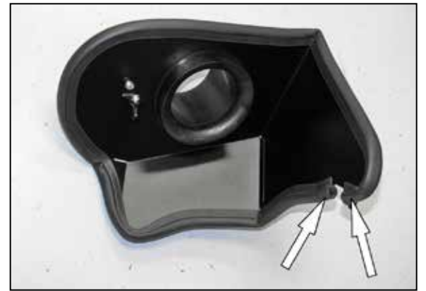
17. Install the provided edge trim onto the heat shield as shown.
