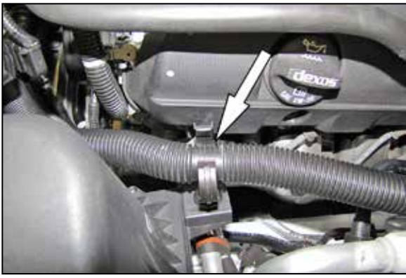
7. Open the clamp securing the sound tube to the air filter housing.
