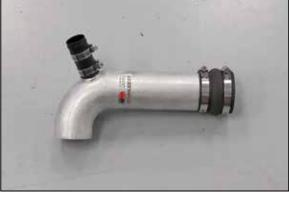
16. Install the remaining coupling hose (08185) onto the  $K\&N^{\otimes}$  intake tube as shown.
