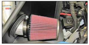
20. Install the K&N<sup>®</sup> air filter onto the intake tube and secure with the provided hose clamp.
