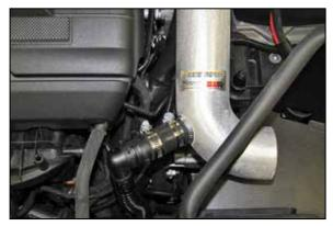
19. Connect the secondary air hose onto the Quick disconnect fitting and connect the vacuum line to the fitting installed into the K&N<sup>®</sup> intake tube. NOTE: On vehicles not equipped with a secondary air tube, install the provided cap into the fitting installed on the K&N<sup>®</sup> intake tube.
