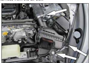
10. Remove the two bolts that secure driver side air box and loosen the hose clamp to the intake tube.
