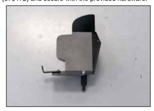
30. Install the provided mounting stud onto the driver's side heat shield and secure with the provided hardware.
