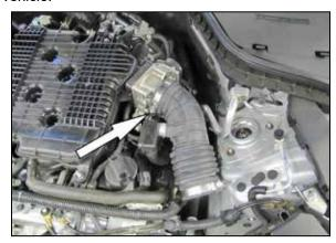
12. Loosen the hose clamp securing the driver's side intake hose to the throttle body.
