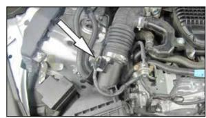
4. Disconnect the Passenger side mass air sensor electrical connection and unhook the wiring harness from the air box.
