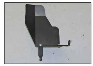
16. Install the provided mounting stud onto the passenger side heat shield and secure with the provided hardware.
