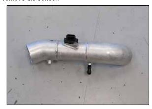
35. Install the mass air sensor into the K&N $^{\circ}$  intake tube and secure with the provided hardware.
