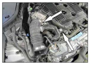
7. Loosen the hose clamp securing the passenger side intake hose to the throttle body and remove the bolt securing the crank case vent to the intake manifold.
