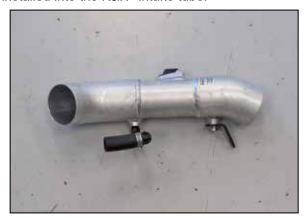
38. Install the tube mounting bracket (070049) onto the  $K\&N^{\otimes}$  intake tube and secure with the provided hardware.
