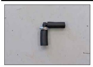
36. Install the 5/8" and  $\frac{1}{2}$ " crank case vent hose's onto the  $\frac{1}{2}$ " 90° fitting.
