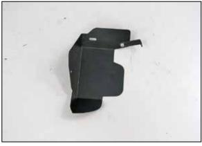
29. Install the heat shield mounting bracket (070109) onto the driver's side heat shield (073172) and secure with the provided hardware.
