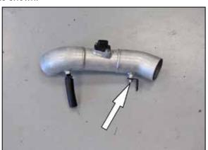
24. Install the tube mounting bracket (070066) onto the passenger side K&N<sup>®</sup> intake tube as shown but do not completely tighten at this time.
