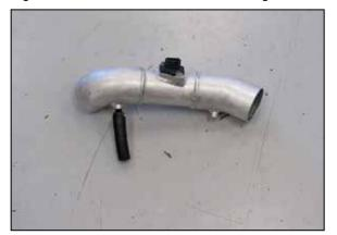
23. Install the 3-1/4" long section onto the fitting installed into the passenger side  $K\&N^{\otimes}$  intake tube as shown.
