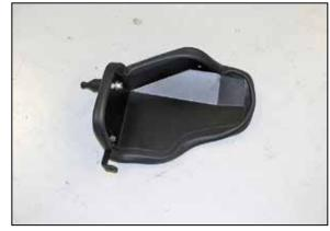
17. Install one of the provided edge trim pieces onto the passenger side heat shield as shown.
