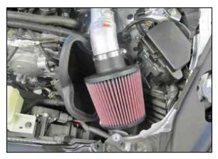
40. Install the K&N® air filter and secure with the provided hose clamp. Adjust the intake tube, heat shield and filter for pest fit and then secure all of the mounting points.
