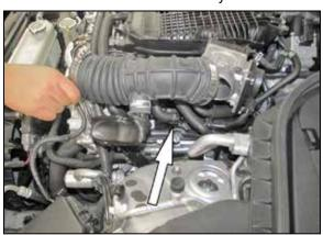
13. Pull the intake hose up to gain access to the crank case vent to valve cover connection. Release the clamp securing the crank case vent and then remove the driver's intake hose assembly.
