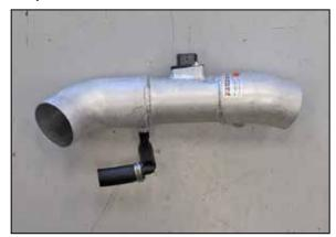
37. Install the vent assembly onto the vent fitting installed into the  $K\&N^{\otimes}$  intake tube.
