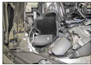
32. Install the heat shield into position as shown on the driver side frame rail and then secure to the core support with the provided hardware.
