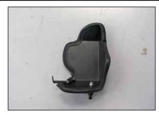
31. Install one of the provided edge trim pieces onto the driver's side heat shield as shown.
