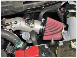
21. Install the  $K\&N^{\odot}$  air filter onto the intake tube and secure with the provided hose clamp.
