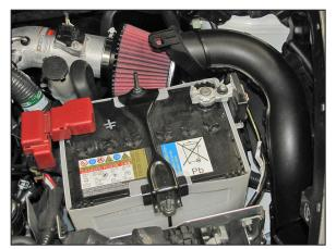
23. Reinstall the fresh air intake tube as shown.
