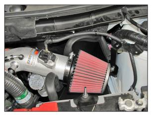
22. Route the mass air sensor wiring harness around the rear of the heat shield and then connect the mass air sensor electrical connection.
