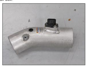
16. Install the mass air sensor into the K&N $^{\! \rm 8}$  intake tube and secure with the provided hardware.
