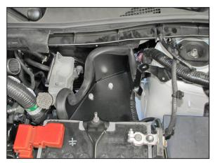
12. Install the heat shield into position on the air box mounting grommets as shown.
