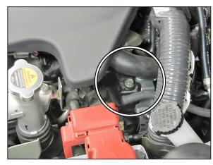
17. Remove the 6mm cover bolt shown.
