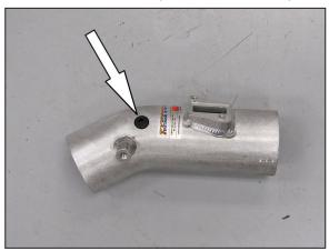
14. Install the provided grommet into the K&N® intake tube as shown.
