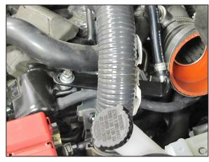
18. Install the tube mounting bracket (083164) onto the location from step #17 and secure with the provided hardware.
