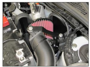
24. Secure the fresh air intake tube with the provided bracket (064315) and hardware on top of the heat shield mounting bracket.
