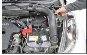
4. Pull up and release the fresh air intake tube and then remove the fresh air intake tube from the vehicle.
