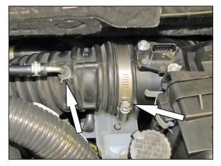
3. Loosen the hose clamp securing the intake hose to the air box and then release the spring clamp securing the turbo waste gate vent line to the intake tube.
