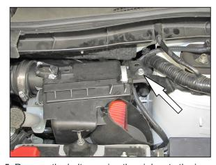
5. Remove the bolt securing the air box to the inner
