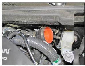
13. Install the coupling hose (5-1045) to the turbo inlet and secure with the provided hose clamp.
