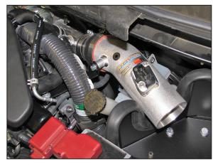
19. Install the K&N® intake tube into the coupling hose at the turbo inlet and align with the mounting bracket. Then secure the intake tube with the provided hardware and hose clamp.
