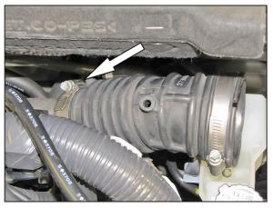
8. Loosen the hose clamp securing the intake hose to the turbo inlet and then remove the intake hose from the vehicle.
