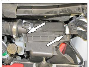
6. Release the two air box retaining clips and then remove the front half of the air box housing from the vehicle.
