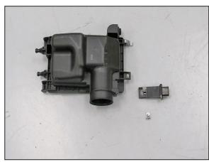
15. Remove the mass air sensor from the factory air box.
