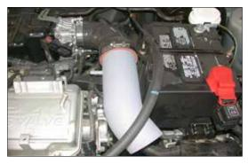
15. Install the Typhoon intake tube into the silicone hose as shown.
