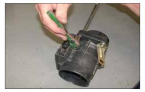
12. Using the provided hardware, secure the provided mass air adapter and the wire harness bracket to the stock mass air sensor as shown.
