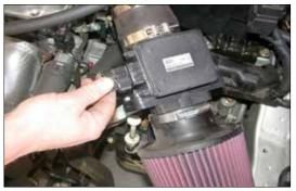
20. Reconnect the mass air sensor electrical connection as shown.
