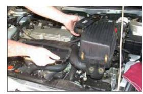
7. Loosen and remove the three bolts that secure the air cleaner assembly, then, remove the air cleaner assembly as shown.
