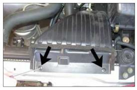
6. Depress the center pins on the air inlet duct as shown.
