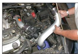
24. On manual transmission vehicles install the cold air intake tube assembly into the vehicle as shown.
