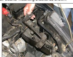
10. Remove the stock air cleaner mounting bracket as shown.
