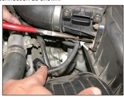
3. Unclip the mass air sensor wire harness from the stock hanger as shown.
