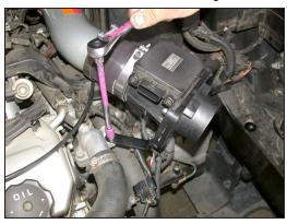
20. Secure the bracket to the water neck using the bolt removed in step 18.
