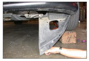
28. On automatic transmission vehicles raise the vehicle up and secure it with jack stands. Now remove the 5 screws that secure the lower valance and pull the valance back as shown.
