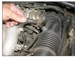
4. Disconnect the crankcase vent hose from the stock intake tube as shown.
