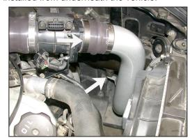
26. Slide the hump hose onto the mass air sensor, then, line up the bracket on the cold air tube with the rubber mounted stud on the bottom of the inner frame rail as shown.
