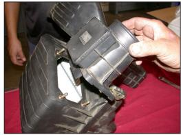
15. Remove the nuts that secure the mass air sensor to the stock air cleaner then, remove the mass air sensor as shown.
