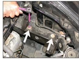
9. Remove the two bolts that secure the stock air cleaner mounting bracket as shown.
