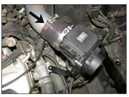
19. Slide the mass air sensor assembly onto the intake tube as shown but do not tighten.
