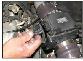
33. Reconnect the mass air sensor electrical connection as shown.
