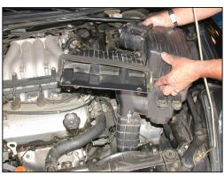
8. Remove the complete air cleaner assembly as shown.
