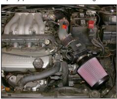
35. This K&N® high flow intake system has been designed to be used in two different configurations. In the case of inclement weather, the cold air tube can be removed and the air filter can be clamped onto the intake tube located in the engine compartment to avoid the possibility of ingesting water into the engine.
