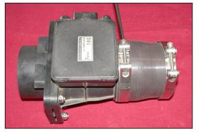
17. Install the silicone step hose and hose clamps onto the mass air sensor and tighten as shown.
