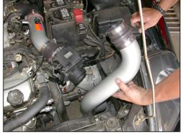
25. On automatic transmission vehicles install the cold air intake tube only as the air filter will be installed from underneath the vehicle.
