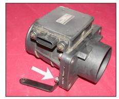
16. Assemble the provided mass air sensor adapter, bracket and the stock mass air sensor and stock gasket using the provided hardware as shown
