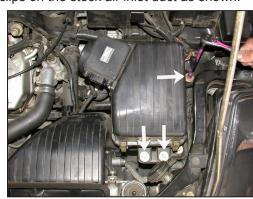
7. Loosen the 3 bolts that secure the air cleaner assembly as shown.
