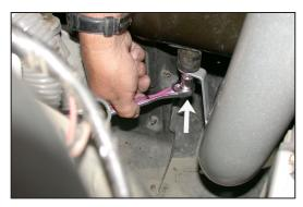
27. Secure the bracket to the rubber mounted stud using the provided hardware as shown.
