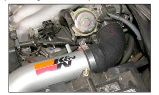
14. Slide the intake tube assembly onto the throttle body as shown but do not tighten.
