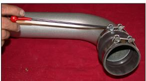
21. Install the silicone hump hose and hose clamps onto the cold air intake tube and tighten as shown. NOTE: Before installing the silicone hump hose, inspect the inside of the tube for any debris, then clean the inside out with water and a towel. Inspect the tube one more time before proceeding to the next step.
