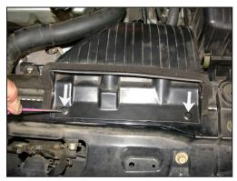
6. Depress the center pins to release the push clips on the stock air inlet duct as shown.
