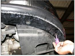
30. Reverse the removal process and re-secure the lower valance as shown.
