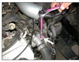
18. Remove the bolt that secures the wire harness to the stock water neck as shown.
