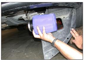
29. From underneath the vehicle install the K&N<sup>®</sup> air filter and secure with the provided hose clamp.
