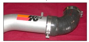
13. Install the silicone hose and hose clamps onto the intake tube as shown but do not tighten.
