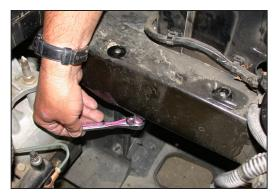
11. Remove the stock bolt on the bottom of the inner frame rail as shown.
