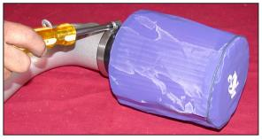
23. On manual transmission vehicles install the  $K\&N^{\odot}$  air filter onto the cold air intake tube and tighten as shown.
